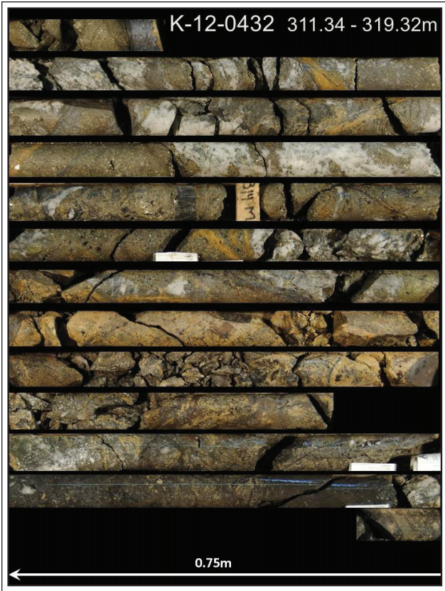
Figure 23. Complete drill hole intercept of K-12-0432 (311.34–319.32 m) showing the quartz and siderite vein types. Composite assay over 6.99 m true width 1180 g/t Ag (37.9 oz/t), 1.5 g/t Au, 2.1% Pb, 7.5% Zn.
