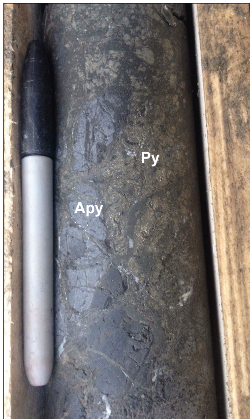
Figure 17. Mineralized sulphosalt + pyrite + arsenopyrite vein at the Rex deposit. Diamond drill hole DG17-955C 129 m. Core diameter is approximately 5 cm.
