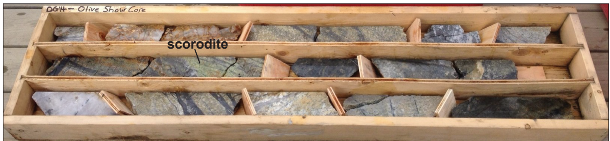
Figure 15. Mineralized quartz-arsenopyrite vein intersections at the Olive zone. Greenish mineral is scorodite. Veins are emplaced into Mayo suite granodiorite. Core diameter is approximately 5 cm.
