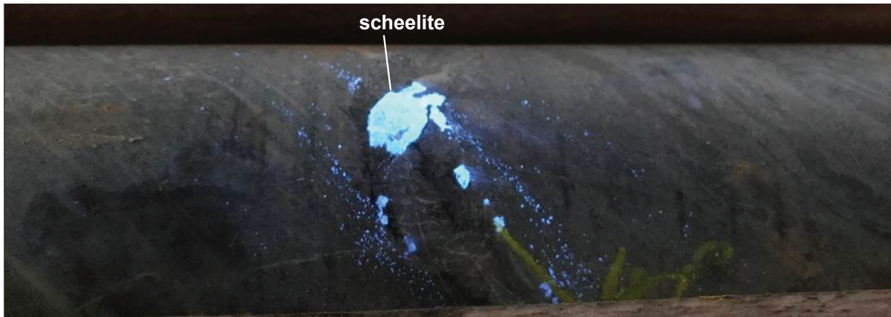
Figure 16. Scheelite (fluorescent mineral) within a skarn horizon in the Mar tungsten deposit. Diamond drill hole DG17-967C 119.6 m. Core diameter is approximately 5 cm.
