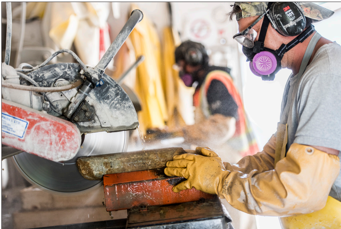
Core cutters at work. Photo courtesy of Yukon Mining Alliance.
