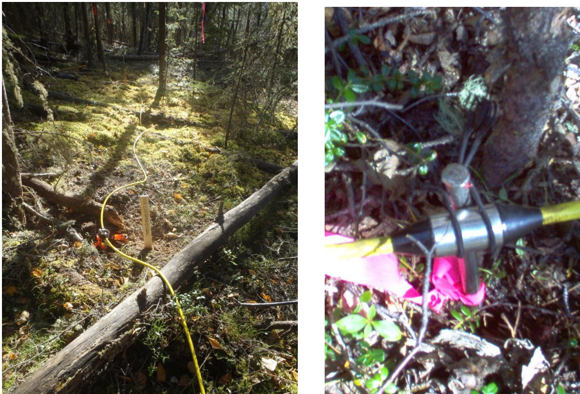
Figure 4. Multi-electrode laid along profile (left) and electrode connected to cable (right).
