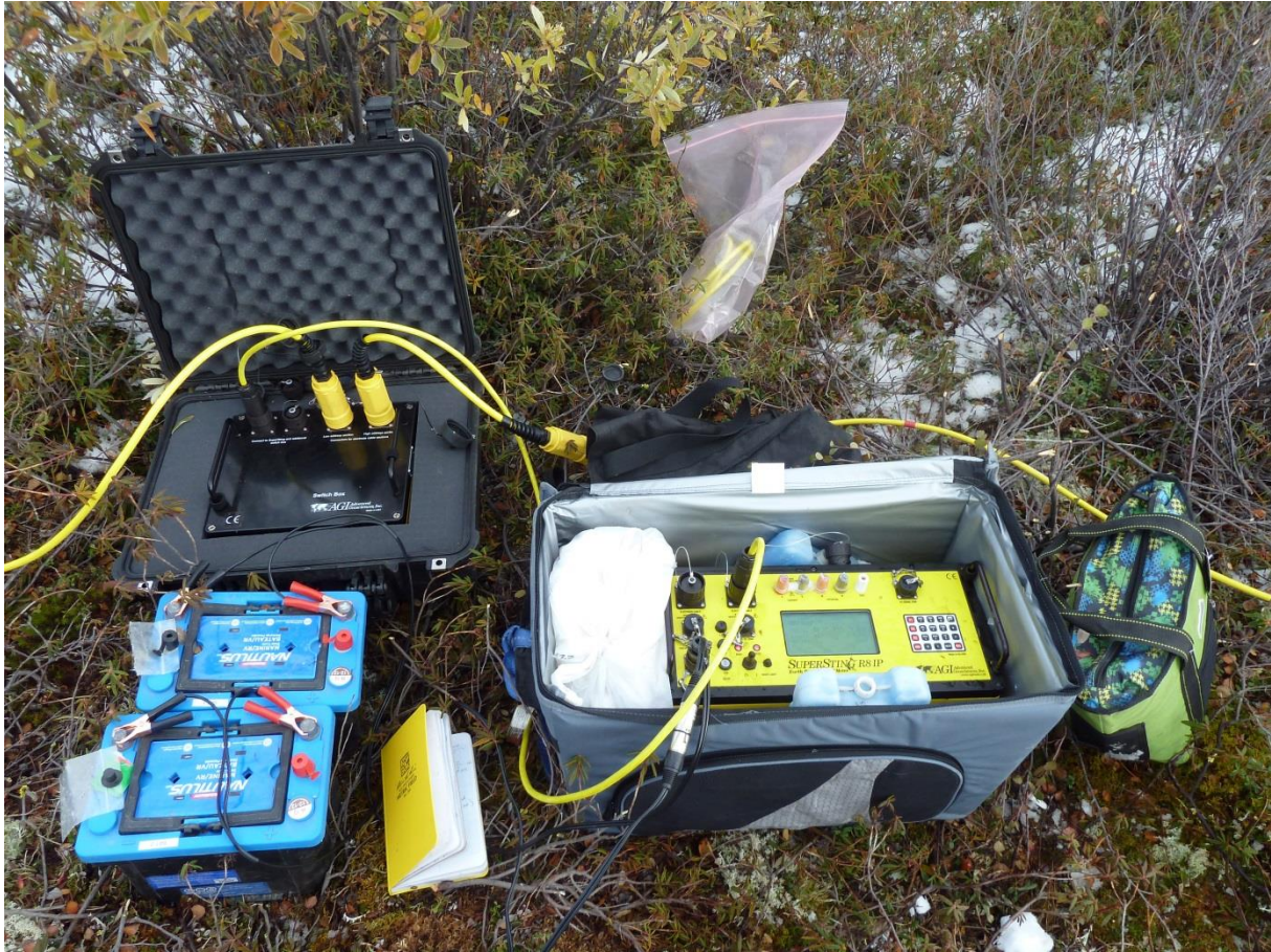
Figure 2. AGI Supersting R8 system console (right), switchbox (upper left), and battery power source (lower left).
