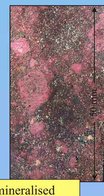
Main ore type: mineralised matrix-supported breccia with clasts of hematitic K-feldspar-altered metavolcanic rock. Matrix is composed of finely disseminated magnetite, pyrite, chalcopryrite and biotite. Photo by G. Mark.
