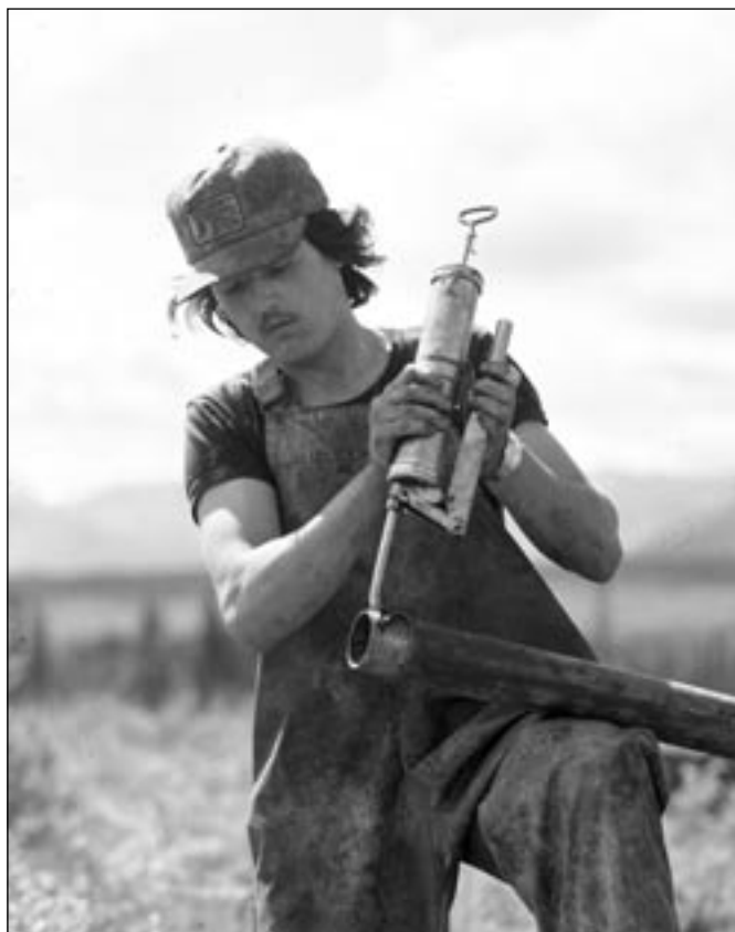
Mining exploration crew member greasing the ends of a drill rod.
