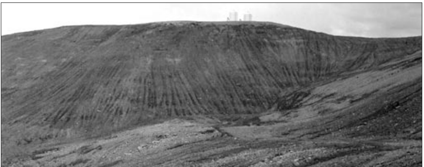
Waste rock at Brewery Creek was smoothed, re-contoured and seeded. In a few seasons, natural vegetation will colonize the disturbed areas.
