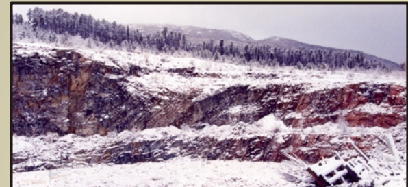
War Eagle North: sedimentary beds dip towards the south at left; red iron oxide alteration at right.
