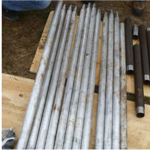
Figure A3. Photograph of aluminum rods used for the Winkie drill for permafrost coring.
