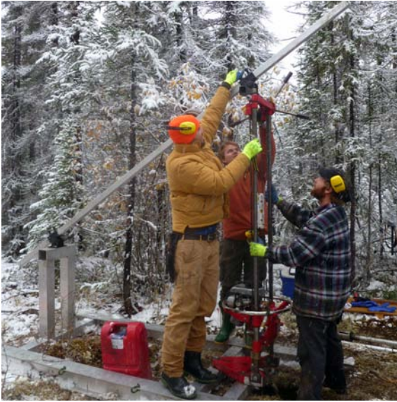
Figure A2. Photograph of the Winkie drill, used for permafrost coring.
