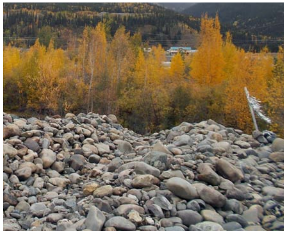
Figure 37. Coarse-grained gravel containing cobbles and pebbles compose dredge tailings, making them unusually porous and subject to high rates of groundwater movement.
