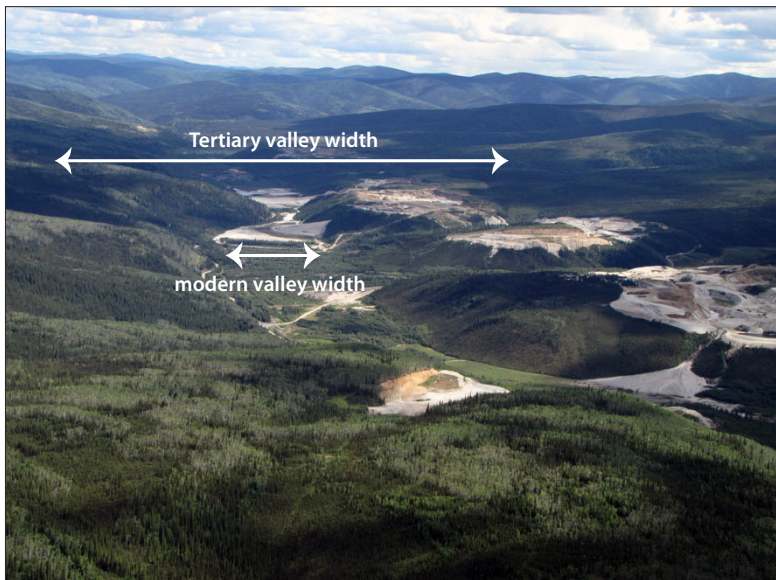
Figure 19. Photo looking south toward the headwaters of Hunker Creek showing the broad valley floor of the Tertiary fluvial system (benches currently being mined) and the narrow, inset valley of the modern Hunker Creek drainage. White Channel gravel is a distinctive deposit that makes up benches up to 100 m above modern stream levels.
