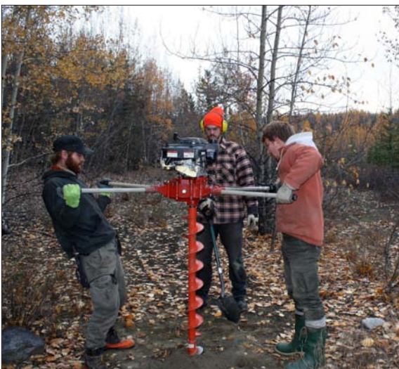
Figure A4. Photograph of the Honda drill, used for permafrost coring.
