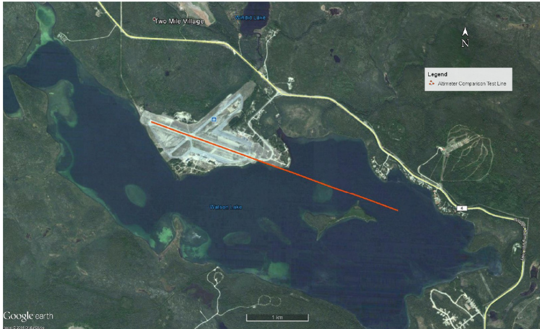
Figure 18: Altimeter Comparison Test Line Location Superimposed on Google Earth
