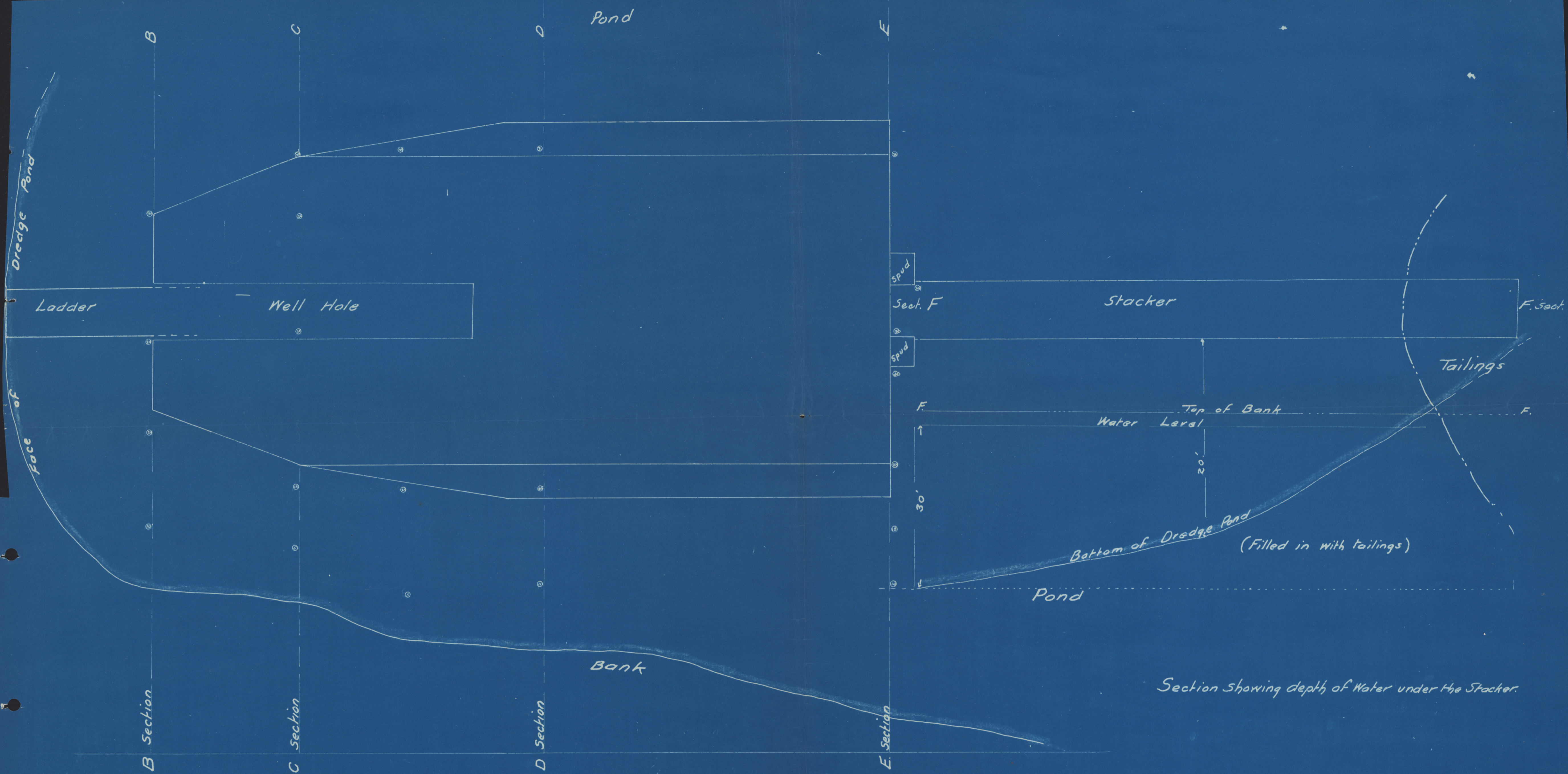
Plan section of Dredge Canadian No 4 Scale 10ft. = 1 inch
