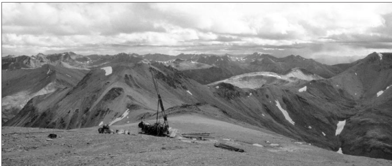
Figure 11. Eagle Plains Resources conducted helicopter-supported diamond drilling on the Fire property in the Pelly Mountains volcanic belt.
