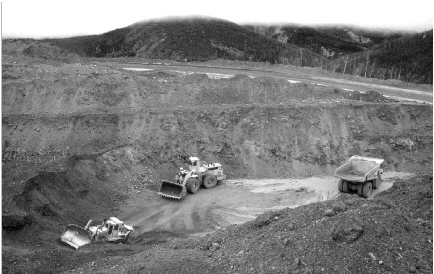
Figure 5. Mining operations at the Moosehead open-pit. Brewery Creek produced ore from four open pits in 2000.
