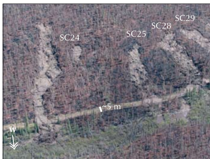
Figure 14. Oblique aerial photograph of multiple active-layer detachments on a west-facing slope. The failures crossed local access trails and deposited material directly into Steele Creek.
