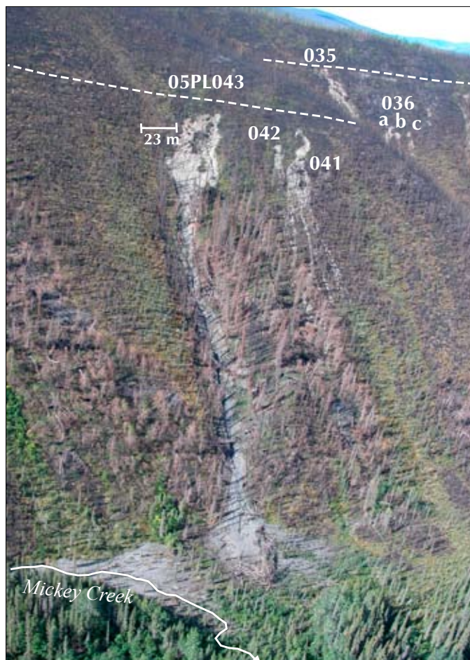
Figure 5. Oblique aerial photograph of numerous failures originating along the scarp of a Pre-Reid glaciofluvial terrace (see dotted lines) on upper, northeast-facing slopes. View is to the southwest. Numbers represent active-layer detachments surveyed near Mickey Creek.
