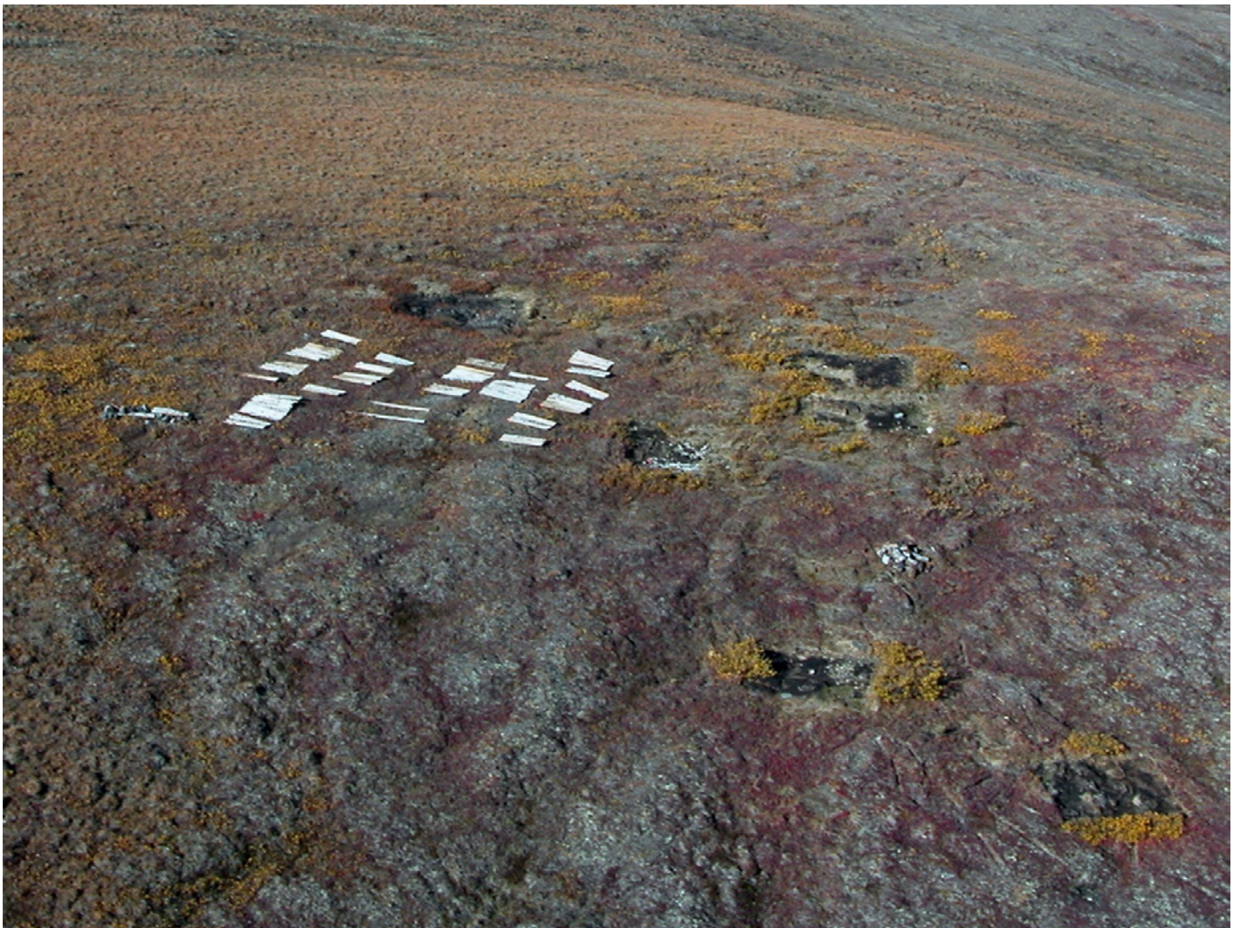
Figure 2. Reclamation and restoration of an abandoned camp site from the 1970s. Black areas show where tent frames were burned. All that remains on-site is core (core boxes are shown in middle of photo).
