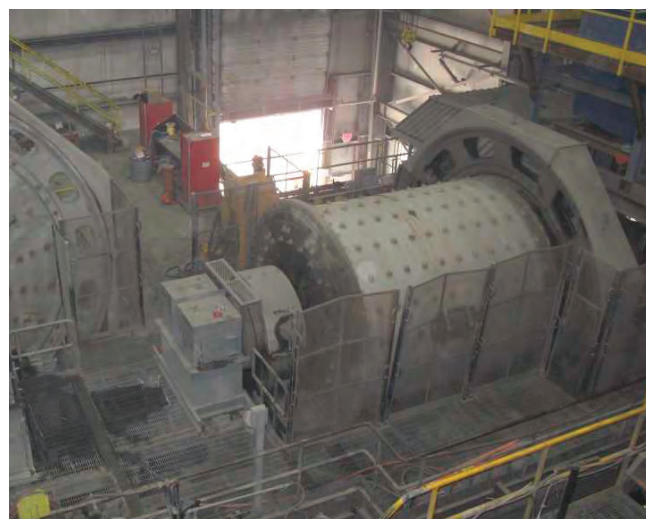
Figure 6. Ball mill at Minto mine.
