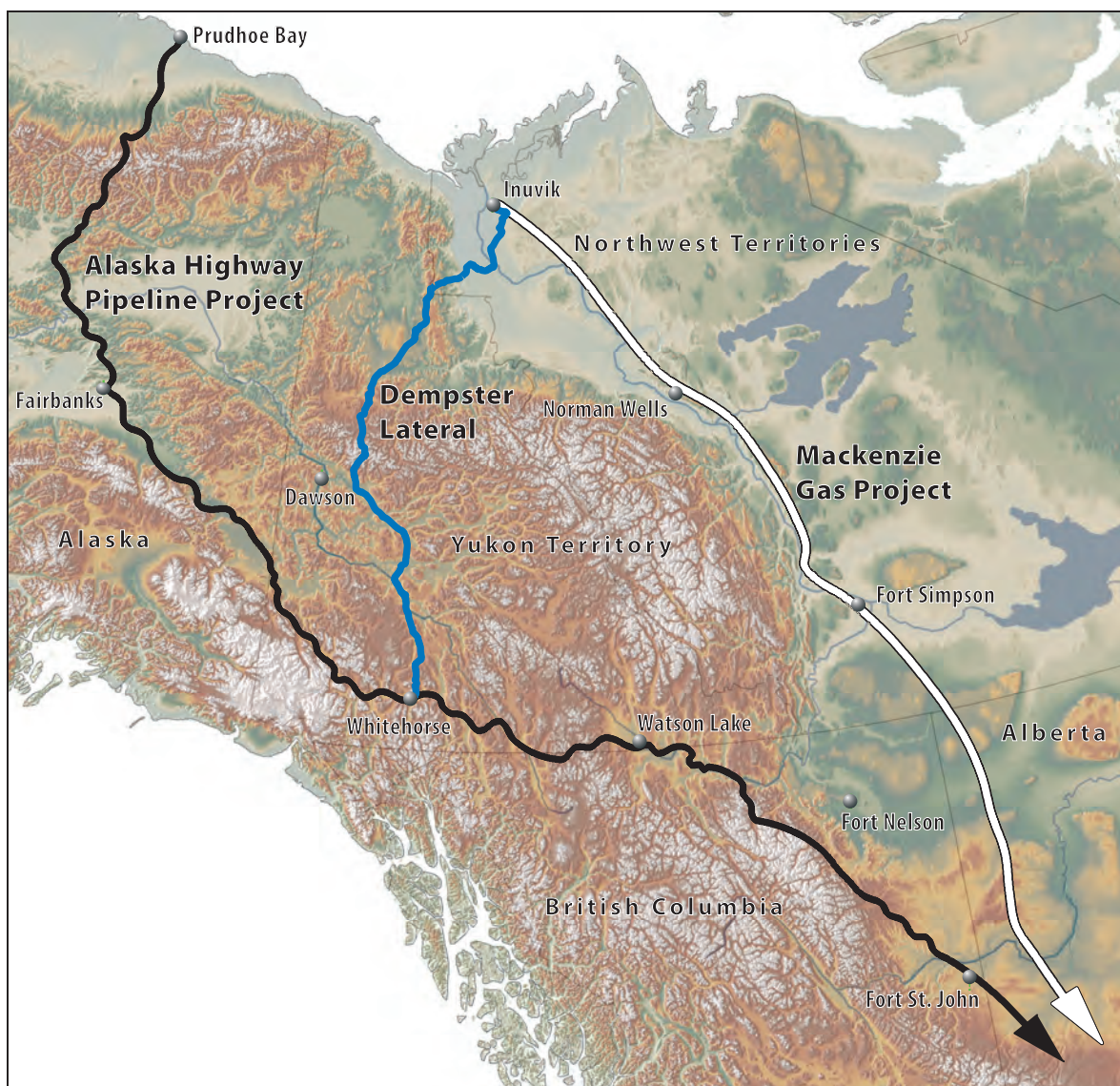
Figure 3. Northern natural gas pipeline options.
