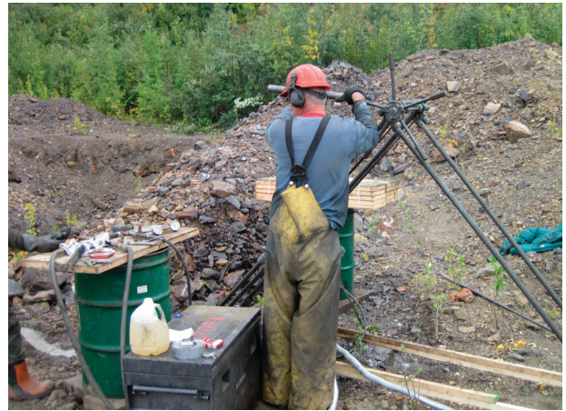
Figure 16. Driven Capital Corp winkie drilling the Lyn property.
