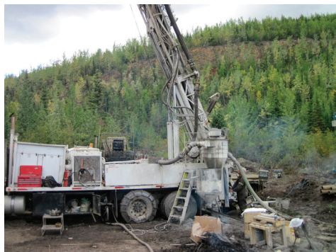
Figure 30. Reverse circulation percussion drilling at Golden Predator’s Grew Creek gold property.
