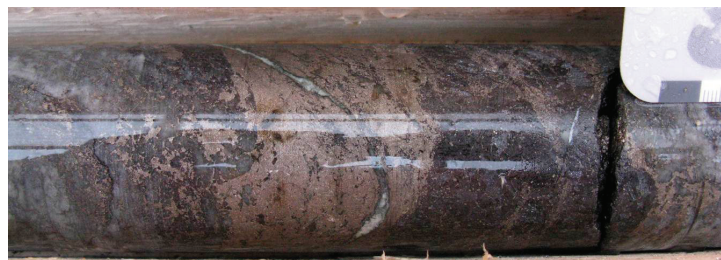
Figure 14. Massive pyrrhotite in drill core from the Keg Main zone of Silver Range Resources.
