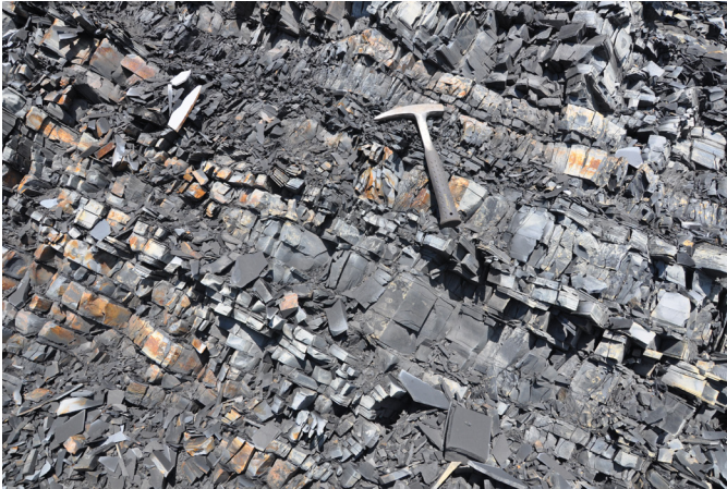
Figure 7. Mudstone and shale lithofacies. Mudstone intervals are thicker and more resistant than shale intervals, and weather into blocks. Shale in this section is <10% and forms thin (<1 cm) partings between blockier mudstone beds. Rock hammer for scale.
