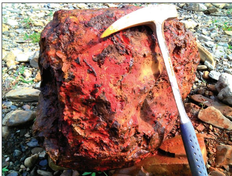
Figure 14. Massive realgar float boulder from Cantex Mine Development Corporation claims in Selwyn basin (photo credit: Cantex Mine Development Corp.).
