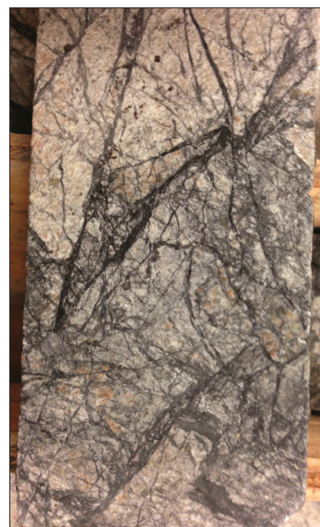
Figure 23. Brecciated drill core from Comstock Metals' QV property. This sample graded greater than 4 g/t Au. Photo courtesy of Comstock Metals Ltd.
