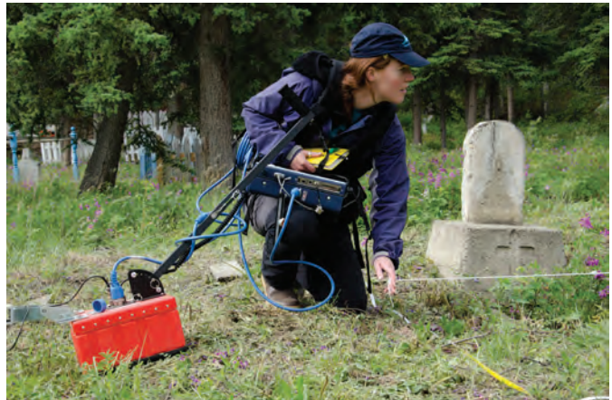
Figure 10. Sarah Laxton collecting GPR data over a grave site.
