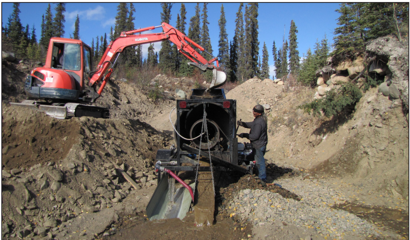
Nick Sawrenko and Charlie Brown using a #10 Gold Machine and a 121-3 Kubota excavator to test the left-limit bench deposit on Florence Creek.
