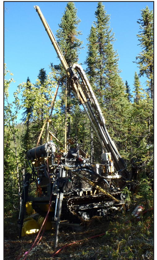
The RAB, a lightweight drilling rig, on-site.
