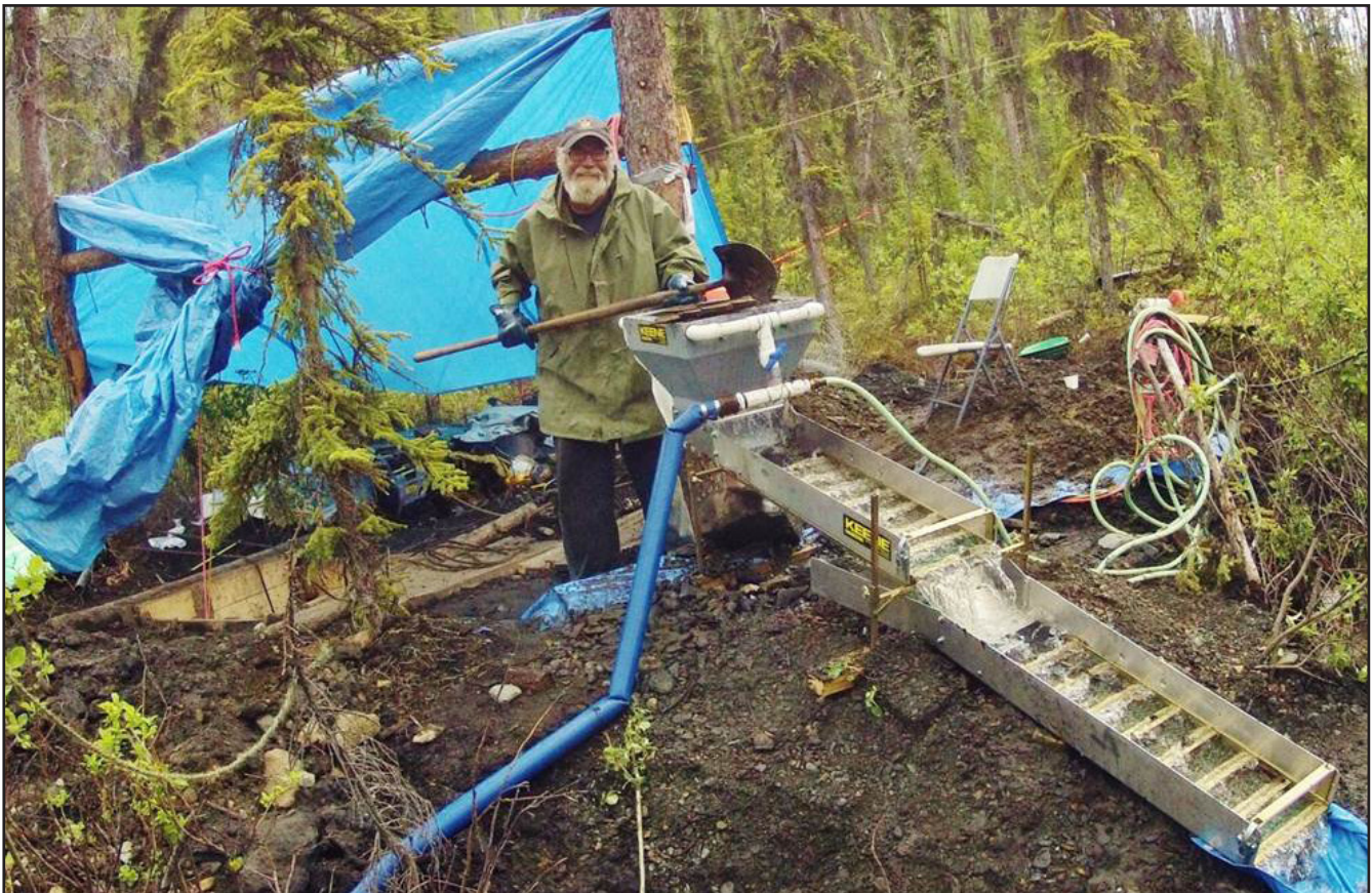
Washing samples from the exploration shaft on Laura Creek. The shaft is visible under the tarp.
