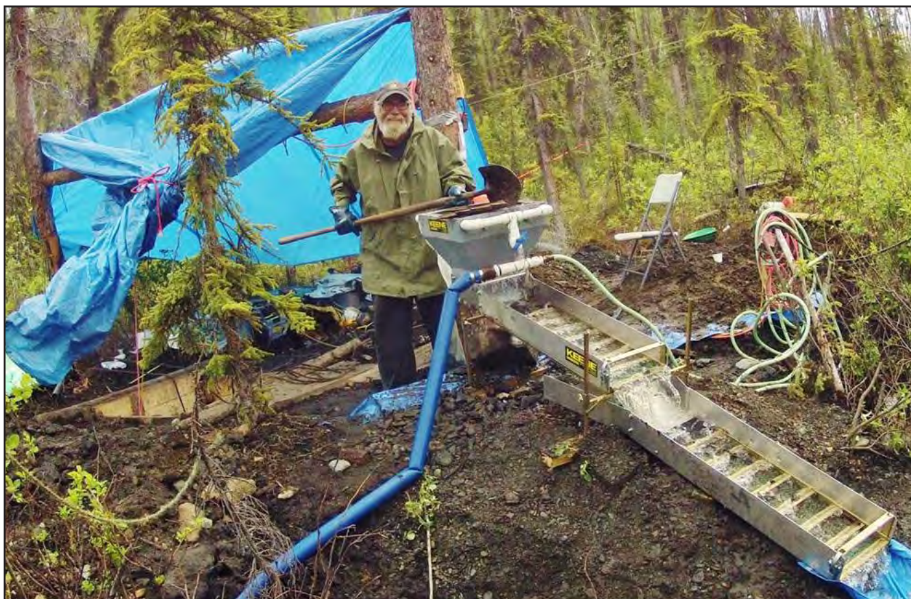
Washing samples from the exploration shaft on Laura Creek. The shaft is visible under the tarp.
