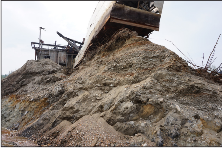
Figure 6. A view of virgin Hunker creek gravel preserved under the tailings stacker of Dredge 11 at the mouth of Last Chance Creek. Tatra Ventures was successful in discovering significant areas of virgin gravel on bedrock in an area that appeared to have been mined out. Their program highlights the potential of working within the dredge limits elsewhere in the Klondike.
