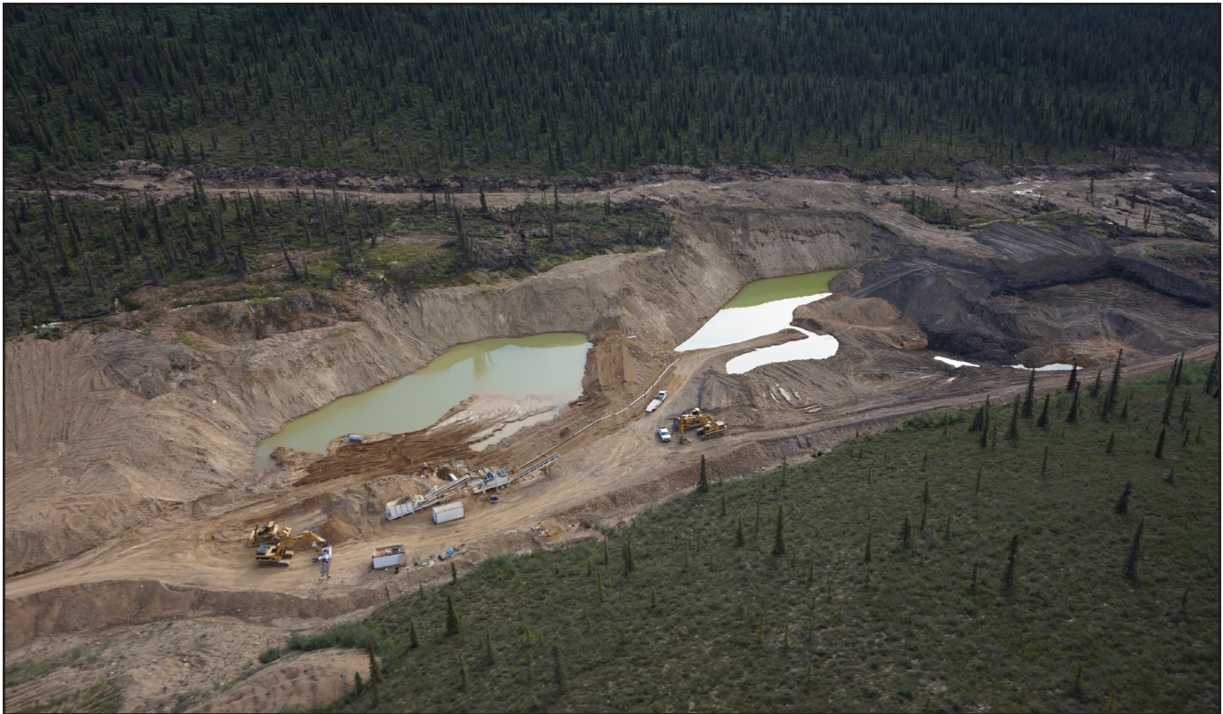
Figure 10. A view to the east over Back Creek in the Mount Nansen mining district. Initial excavations by A-1 Cats in 2015 focused on the left limit searching for a pre-glacial gravel on bedrock under a layer of early Pleistocene till. Remnants of the pre-glacial gravel were discovered closer to the valley center-line and a post-glacial gravel became the mining focus later in the season.
