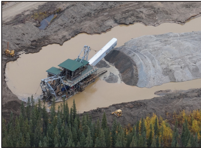
Figure 4. An aerial view of the former Queenstake dredge now operating on the Indian River by Tamarack Inc. Dredging is regarded as one of the more environmentally friendly mining methods, specifically pertaining to fuel consumption, sediment discharge and on-going reclamation.
