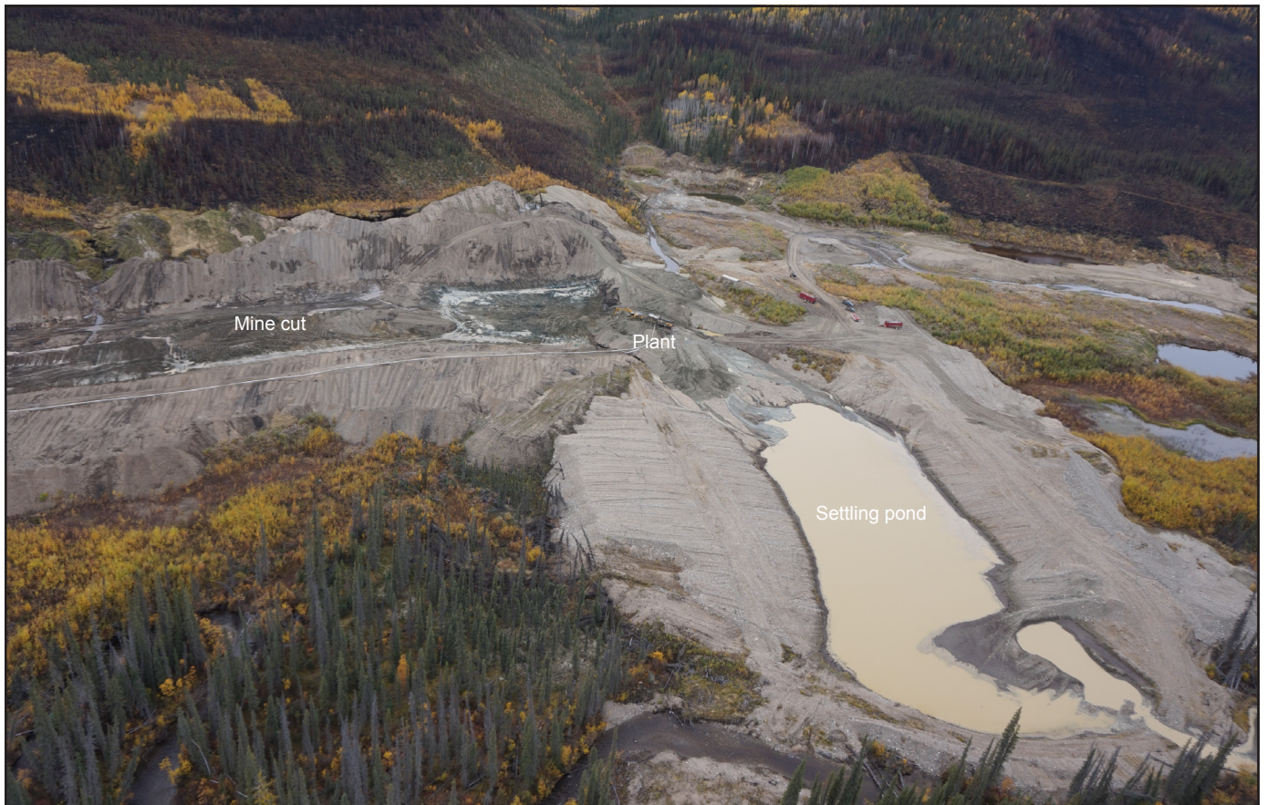
Figure 7. An aerial view of Schmidt Mining's operation on Barker Creek near the mouth of Dixie Creek. Their 2015 cut is located upstream of the old-timer workings on Dixie Bench. The processing plant is located between the mine cut and settling pond.
