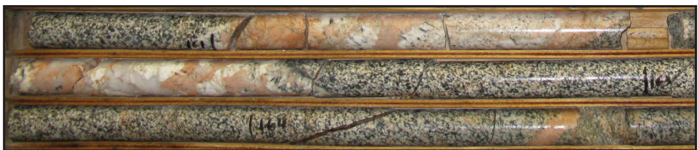
Figure 8. Granitic pegmatite in diamond drill hole 08SWC278 crosscutting unfoliated granodiorite of the Minto pluton. Core diameter is NQ2, 5.7 cm.
