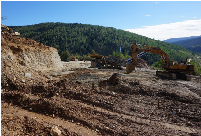
Figure 8. Beron Placers operation on the south rim of Cheechako Hill. A cross cut of the remaining White Channel Gravel was completed in order to evaluate gold grades both vertically and laterally on the bench. The elevated site will facilitate a tiered processing system in 2017.
