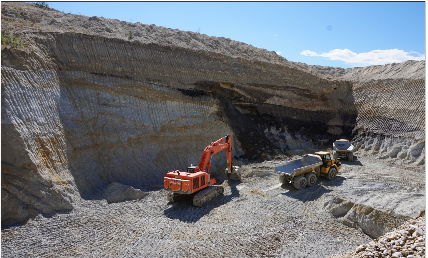
Figure 7. Favron Enterprises cut near the north rim of Dago Hill. The section consists of Paradise gravel overlain by the former soil surface (black organics) and tailings.
