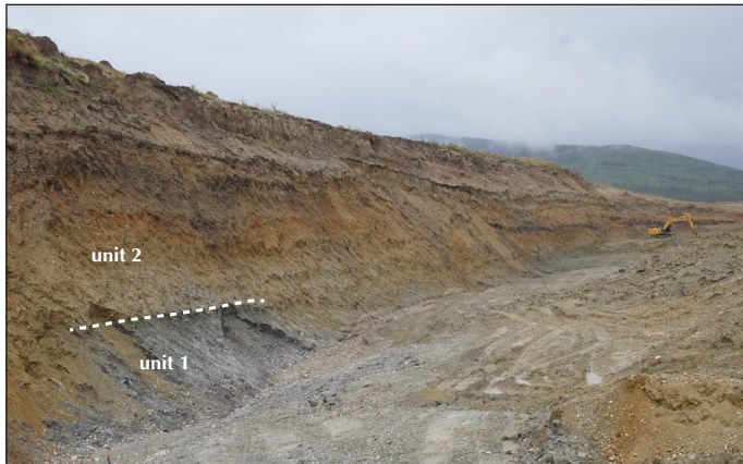
Figure 3. A view looking upstream along the right-limit of the Quartz Creek bench. A greyish gravel (unit 1) is visible near the base of the section. The lower 4.2 m (14 ft) of this unit is considered pay gravel and in places is separated from unit 2 by a woody layer representing a possible depositional hiatus. The section thickness measures 23 m (75 ft).
