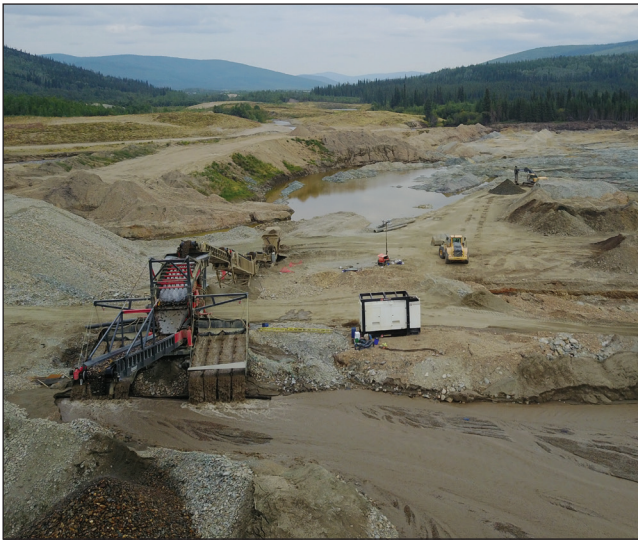
Figure 8. A view of the shaker deck plant and cut at the Little Flake Mine near the mouth of Dominion Creek.
