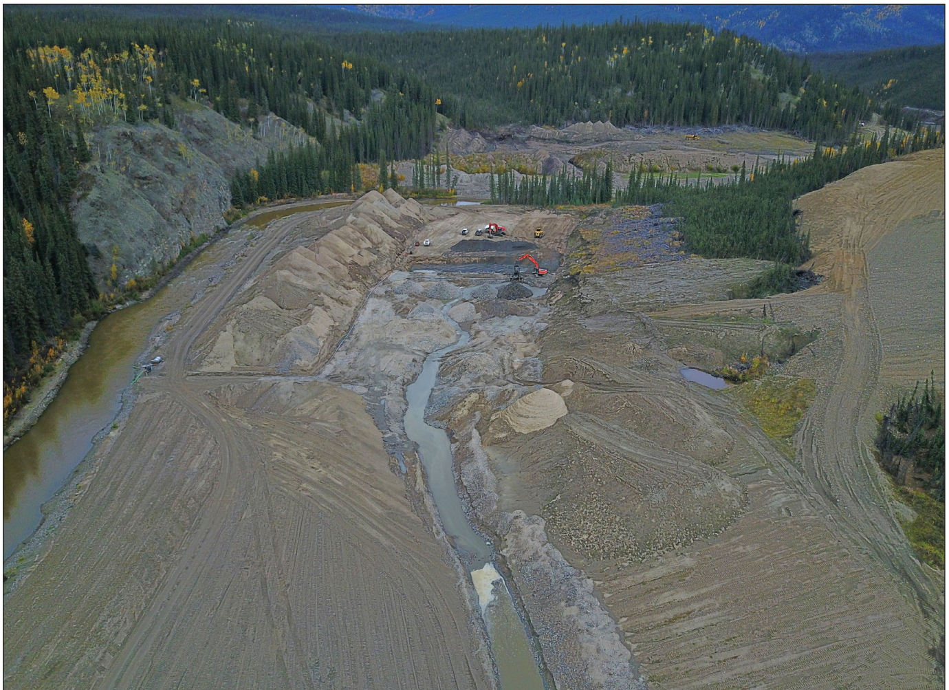
Figure 10. M2 Gold Mines completing their last cut on the flats upstream from camp on the lower Indian River. Reclamation is evident in the foreground and was completed for the entire flat towards the end of the season.
