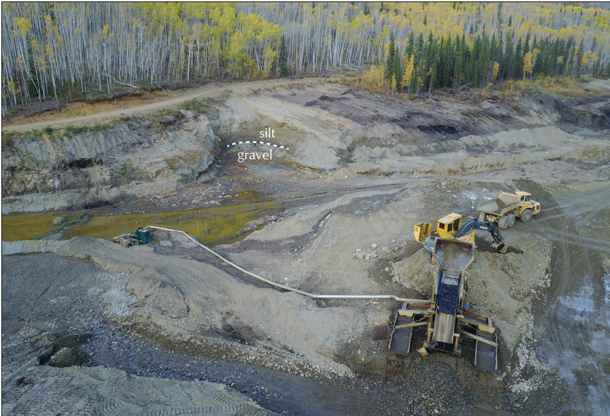
Figure 14. Merrit Sager's wash plant on Kirkman Creek. A test cut into the bank in the background exposed pay gravel buried by silty overburden. The silt buried the floodplain margins between 33,000 and 25,000 years ago at a time heading into cooler conditions associated with the last glacial climate. The silt originates as wind-blown dust (loess) off the nearby Yukon River floodplain. The section is 10.7 m (35 ft) in height.
