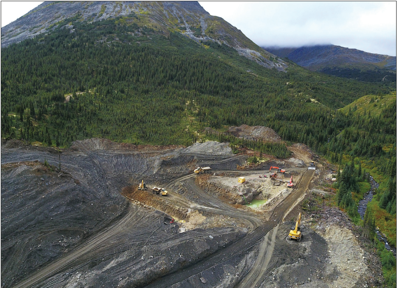
Figure 19. Jim Davies mine on Granite Creek near Keno City. Three Caterpillar 740 haul trucks are used to haul pay to their derocker wash plant.
