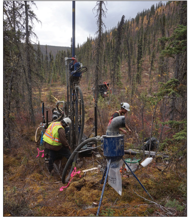
Figure 22. Groundtruth Exploration's heli-portable rotary air-blast drill being used to explore a tributary to Coffee Creek.
