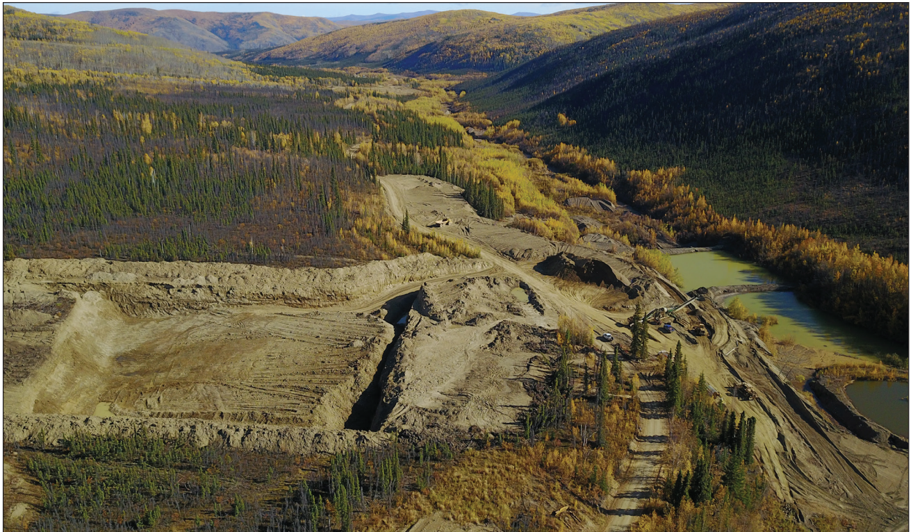
Figure 7. An aerial view looking down the right fork of Eureka Creek. Fine Gold Resources pit is excavated into the left limit Pliocene bench deposit and processed with a trommel in the adjacent valley bottom. The bench deposit underlies the continuous gently sloping surface that extends into the distance.
