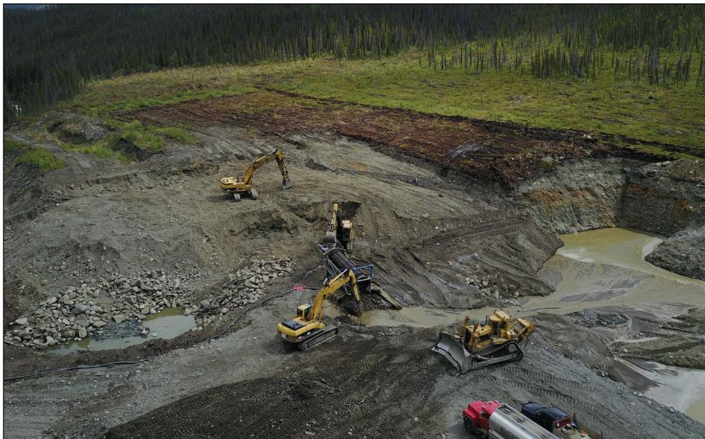
Figure 23. A view of Tic Explorations mine on the left limit of Gladstone Creek. Most mining takes place on low-level gravel bench deposits that lie on a false-bedrock of compact till.
