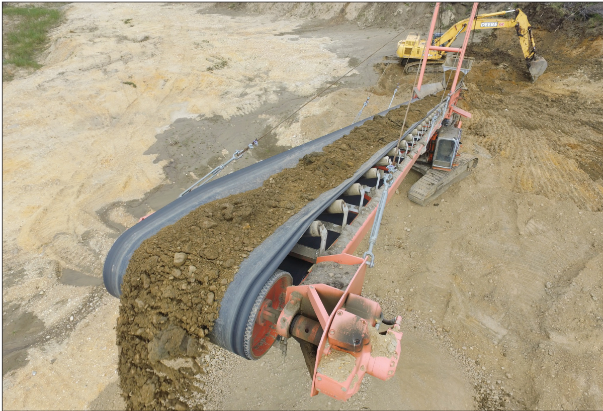
Figure 5. A view looking down on Adrian Hollis' 130 ft excavator-mounted conveyor on Dominion Creek. He has led the evolution of this tool and shares his expertise with other miners on new builds. Photo courtesy of A. Hollis.
