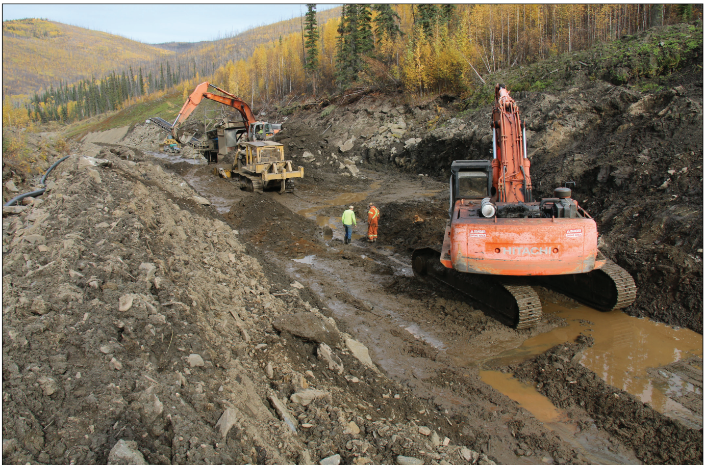
Figure 13. A view of Atlantia Gold Corporations mine on Russian Gulch. Pay gravel from the full width of the valley bottom is being processed for placer gold.
