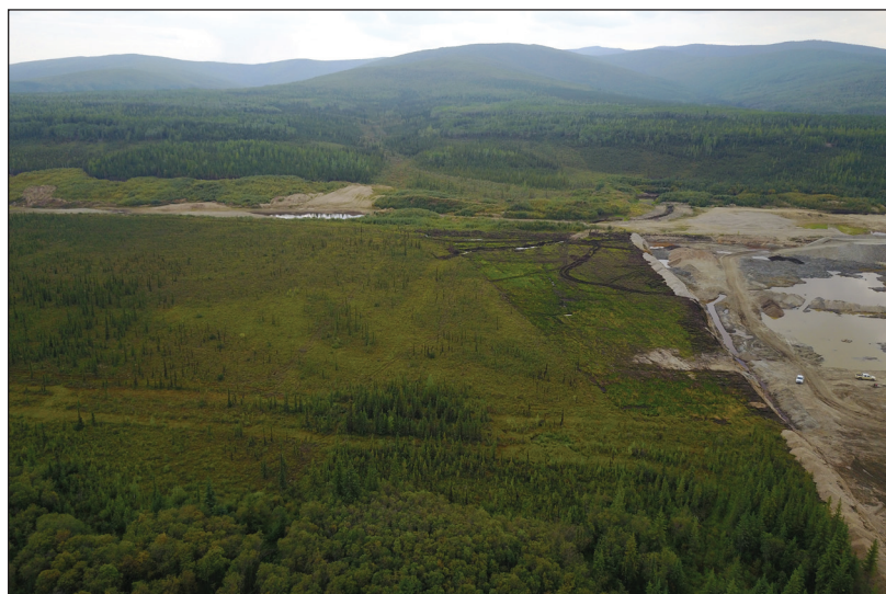
Figure 7. An aerial view over a typical fen wetland near a placer mine in the Indian River valley. The sparsely treed fen wetland is underlain by a layer of reworked loess that is interbedded with organics that accumulated over the last 6,000 years. Permafrost is prevalent. The relatively flat surface is dipping gently towards the foreground allowing surface waters to drain slowly across that landform.
