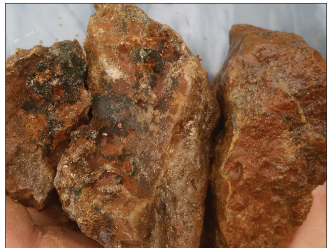
Figure 7. Iron-carbonate altered schist containing trace disseminated pyrite.
