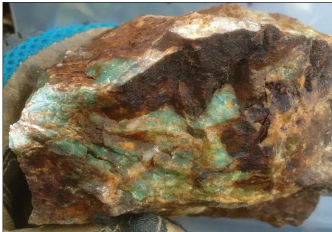
Figure 3. Quartz fluorite breccia cut by vuggy quartz veins and mineralized with trace disseminated pyrite – 0.308 g/t Au.
