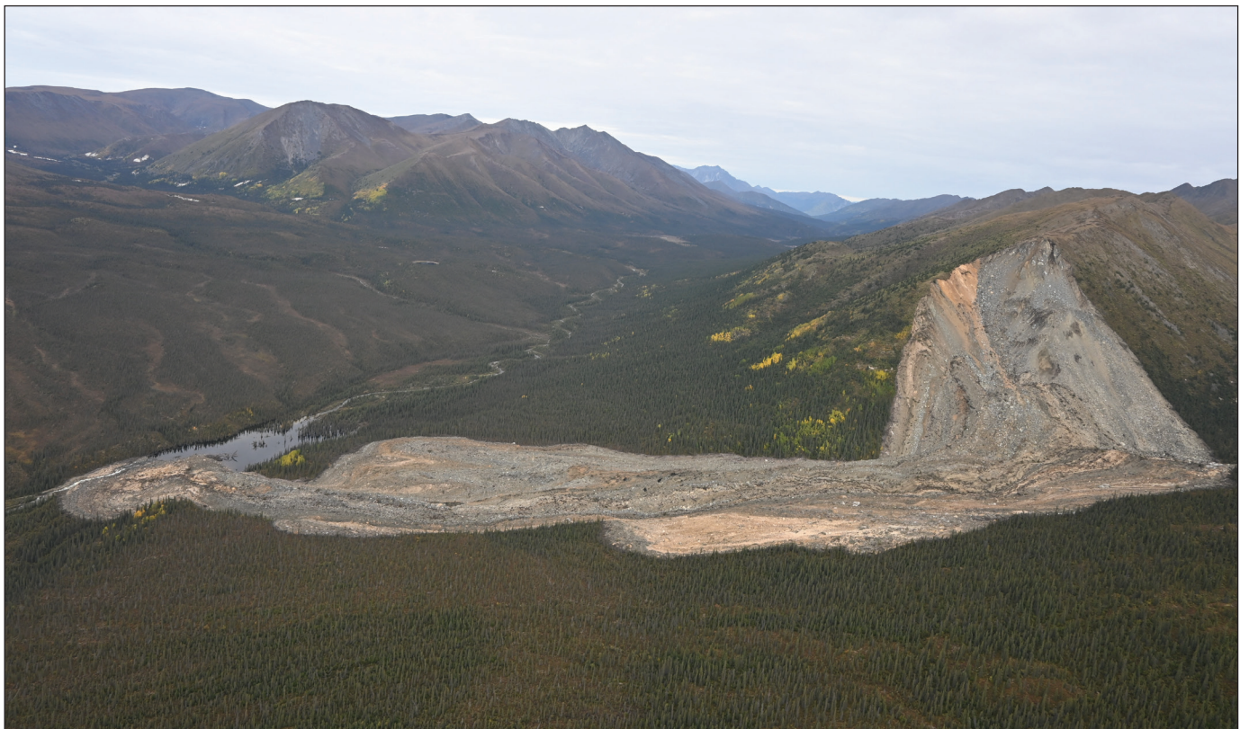
Figure 7. Aerial view of Koidern slide looking northwest along Koidern River valley. Note the accumulation of water upstream from the toe of the slide.
