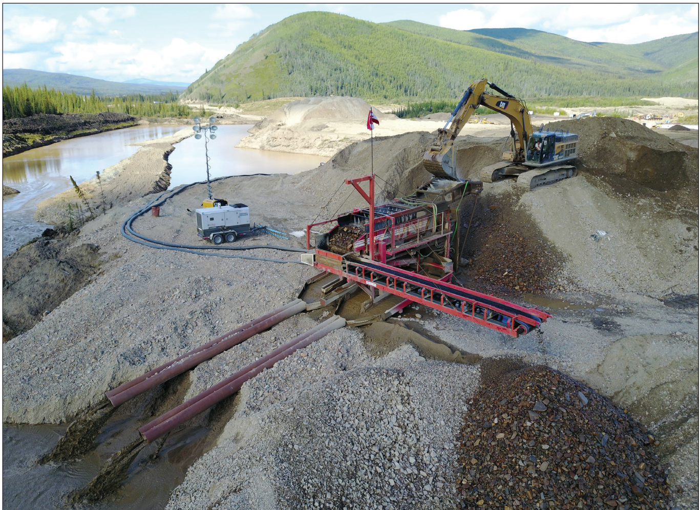
Figure 5. A view of Lonesome Dove Mining's plant on Wounded Moose Creek. A water recirculation system consisting of a long U-shaped settling pond is visible in the background.
