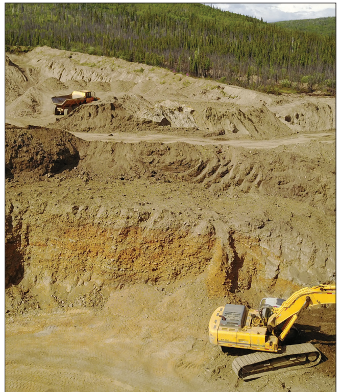
Figure 4. Treadstone Aggregates operation on the Eureka bench. Visible in the foreground is an oxidized pay gravel located on the rim of the bench.
