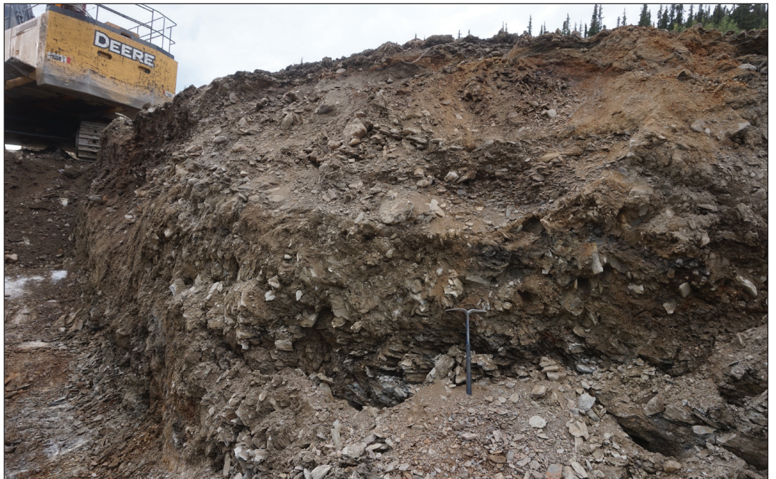
Figure 18. A view of Scott Mining's cut on the right limit of Left Clear Creek. Bedrock is exposed at the base of the cut and two gravel units are present in the cut. The basal, placer gold-bearing gravel is periglacial in origin, deposited during a cold climate. The upper gravel unit is considered a relatively modern gravel and was likely deposited during the current warm period.
