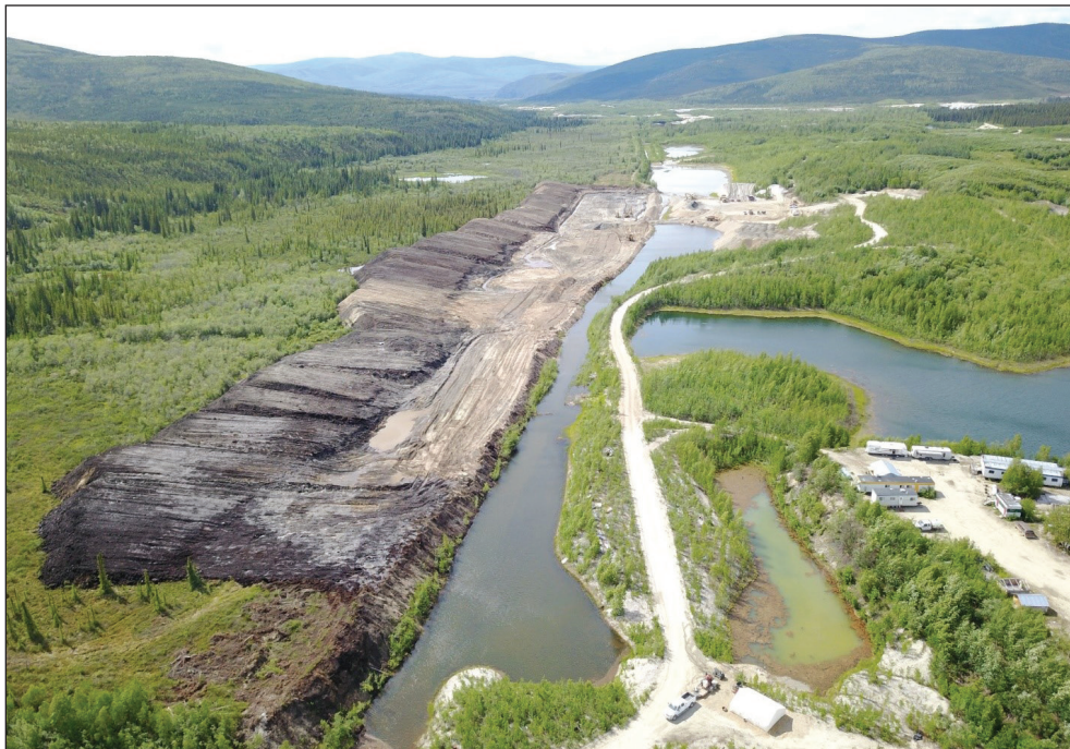
Figure 7. A view over NBC Contracting's operation on Dominion Creek. The Dominion drain is visible to the right of the stripped area. Mining progressed from the downstream end of the property, visible in the distance.
