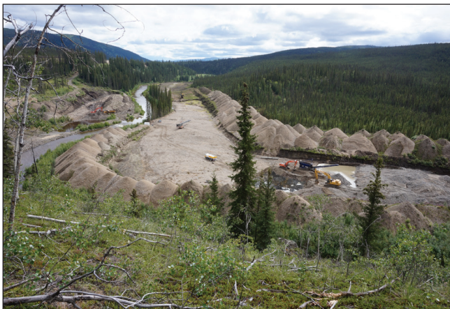
Figure 3. A view looking up the Indian River over Slate River Mining’s operation. Overburden is strategically stacked adjacent to the cut minimizing transport distances and facilitating reclamation.
