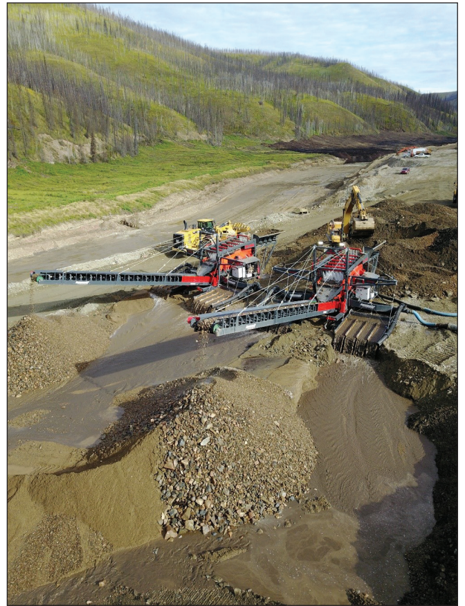
Figure 15. HC Mining added two Macon SD-600 screen deck plants to their operation and had them running side by side later in the season. The plants are fed by a Hitachi ZX470-5 bucket.
