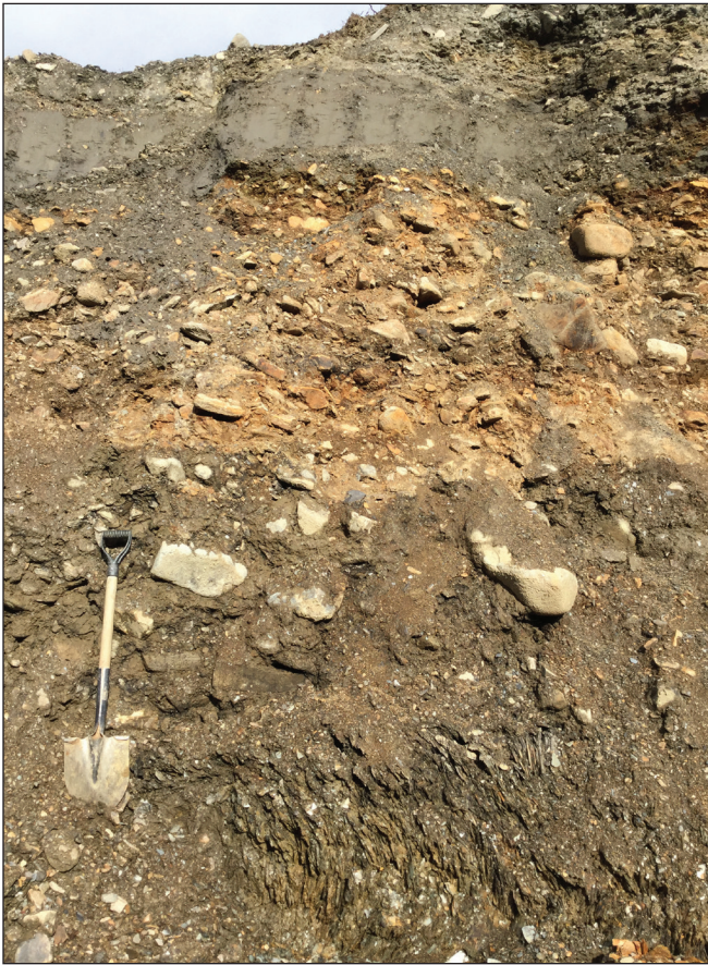
Figure 17. A cut on Josephine Creek shows the schist bedrock overlain by 0.6 m of till, 1.2 m of oxidized gravel and 1 m of silt. The till on bedrock contains the placer gold and was deposited during an early to middle Pleistocene glaciation.
