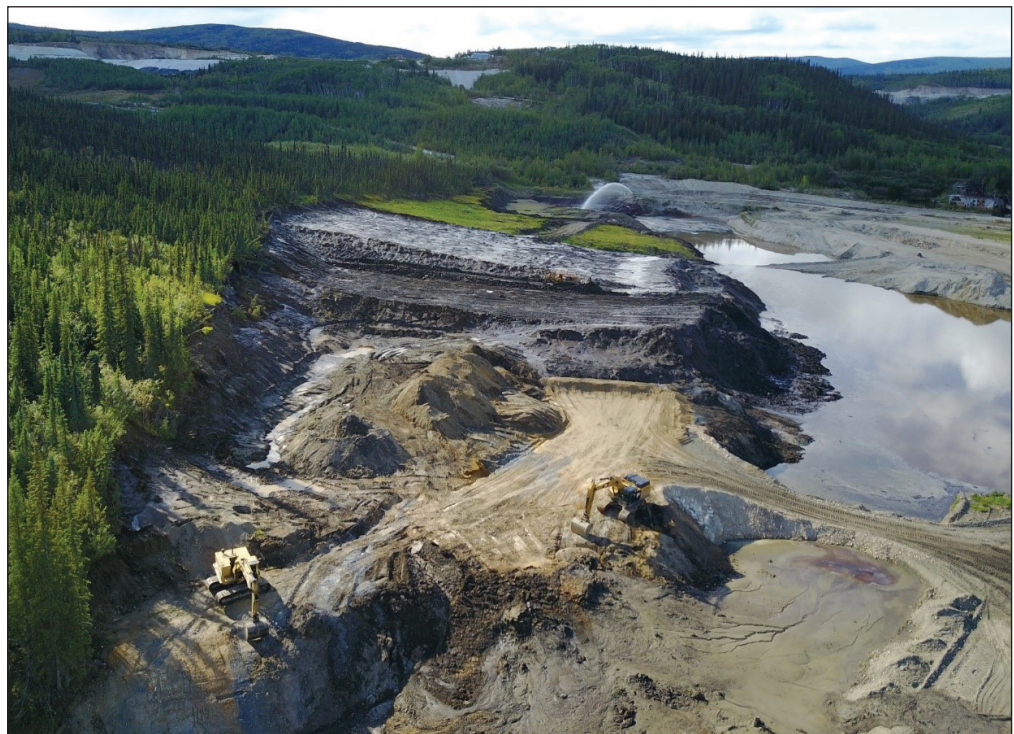
Figure 9. A view to the north looking down the left limit of Hunker Creek near the mouth of Last Chance Creek. The excavators are sitting on a low-level bench, which was the target of operations for the Sailer mine in 2020.
