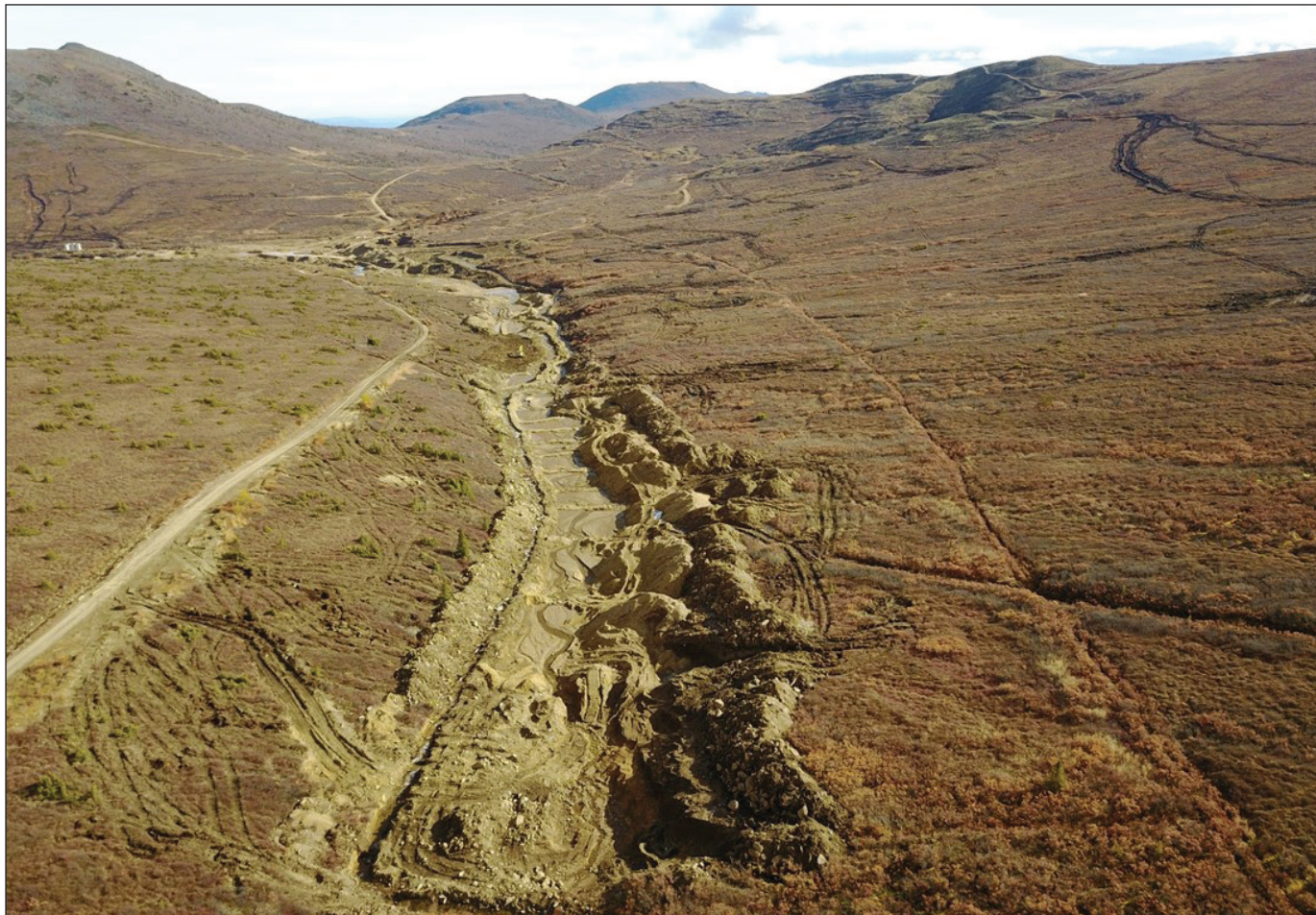
Figure 21. Batavia Mining's operation on upper Canadian Creek near the Casino deposit. Production was focused on the right limit where a low-level bench was encountered.
