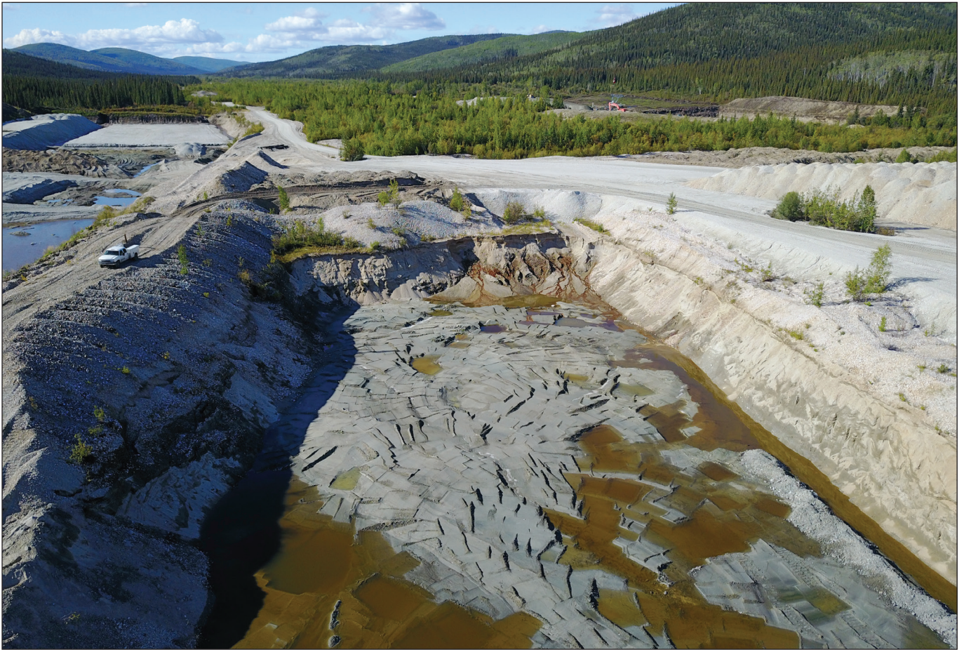
Figure 6. A view to the north of Favron Enterprises dredge tailing cut on Sulphur Creek. Coarse dredge tailings are visible under the pickup truck. Side pay cuts, outside of the dredge limits are also visible in the photo.
