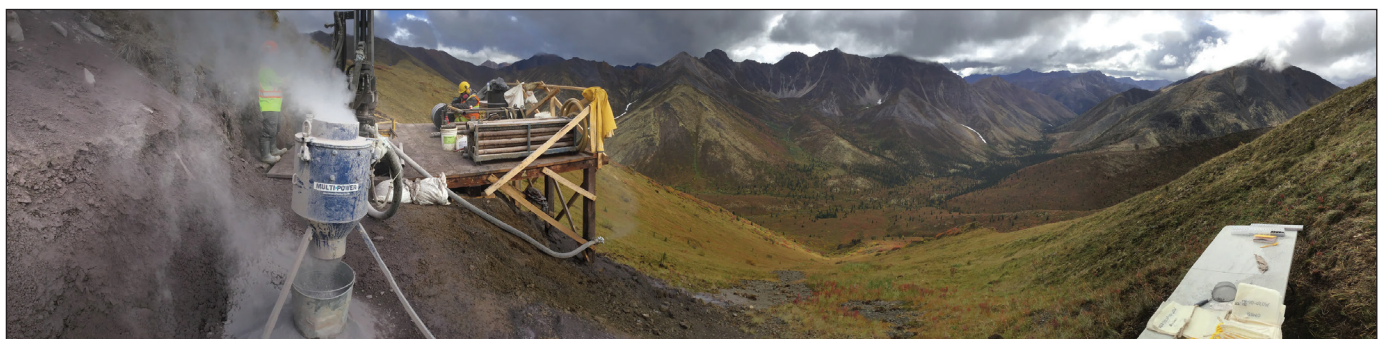
Figure 11. RC drill rig at the Monster IOCG target. Photo from Go Metals Corp. website, accessed November 12, 2020.
