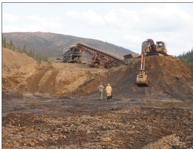
Figure 12. Schmidt Mining processing up to 150 yd 3 /hr on Josephine Creek in 2021.
