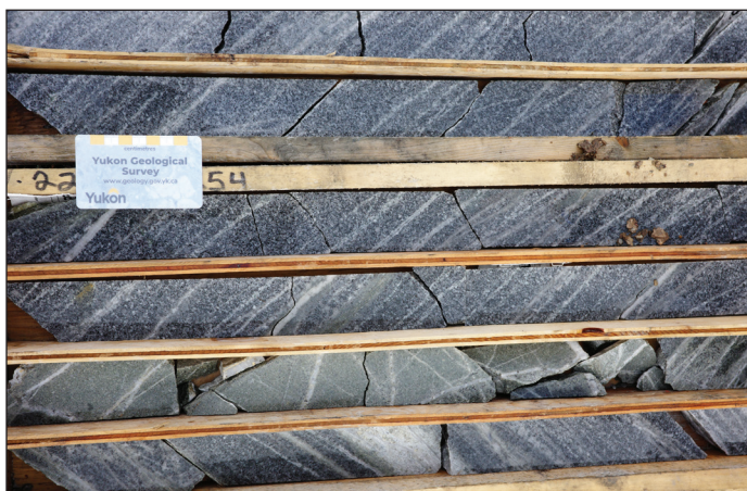
Figure 10. Sheeted gold-bearing quartz veins at in drill core from Snowline Gold's Valley target.
