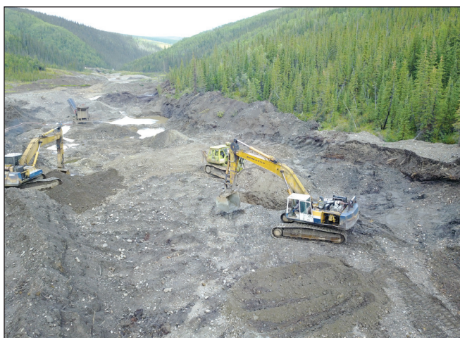
Figure 9. Chrysos Mining processing a low-level, right limit bench deposit on Bruin Creek.
