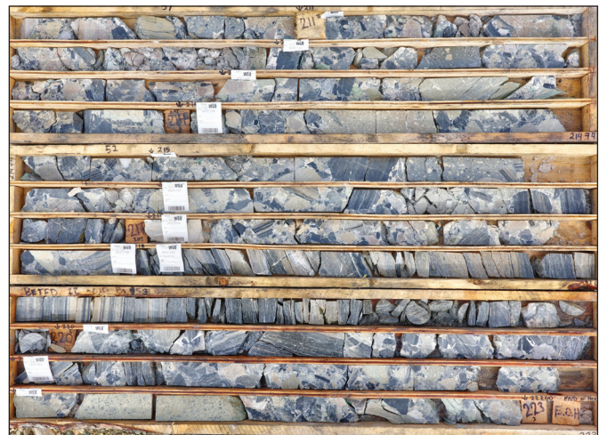
Figure 12. Gold-bearing breccia in drill core from White Gold Corp.'s Betty property.
