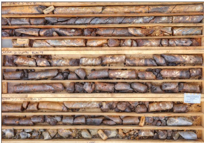
Figure 13. Oxidized manto-style alteration and mineralization in drill core from the Silver Hart property.
