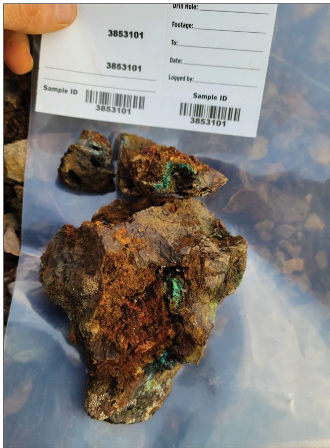
Figure 4. Grab sample from Catch Property containing 7.45 g/t Au and 1.57% Cu.
