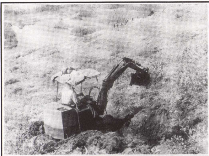
A helicopter-transportable kubota backhoe was used to test coincident geochemical and geophysical anomalies on Noranda's AZ copper-gold skarn property on Hump Mountain north of the White River.
