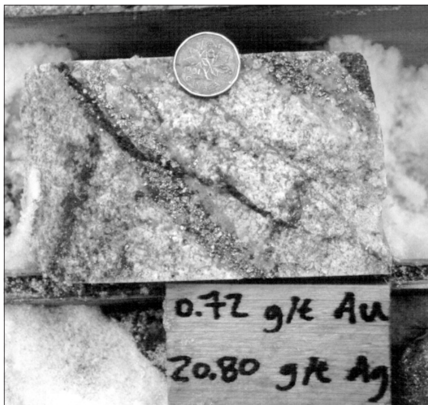
Figure 17. Stringers of pyrite in a clay-altered plutonic breccia from the Porphyry Breccia zone at Mount Nansen.
