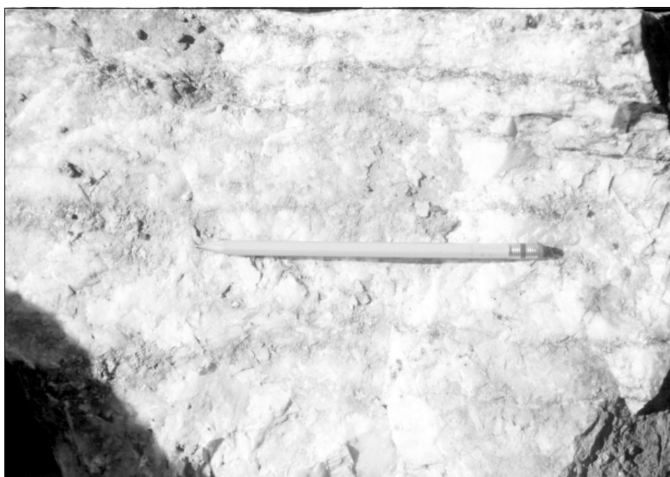
Figure 16. High-grade quartz-sulphide mineralization from the Longline property.
