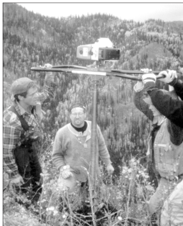
Figure 11. Portable auger drills were used to collect soil samples on the Oki Doki property near Brewery Creek.
