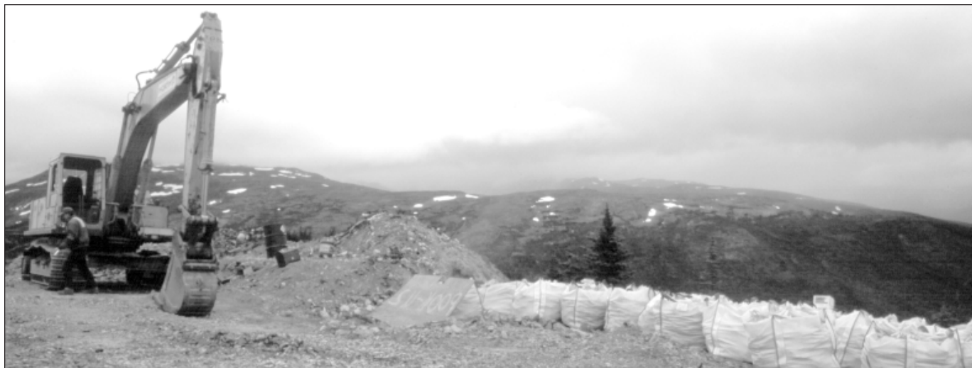
Figure 21. Excavator with loaded ore bags at the Blue Heaven property of Nordac Resources. Each bag contains between 0.9 and 1.5 tonnes of ore.
