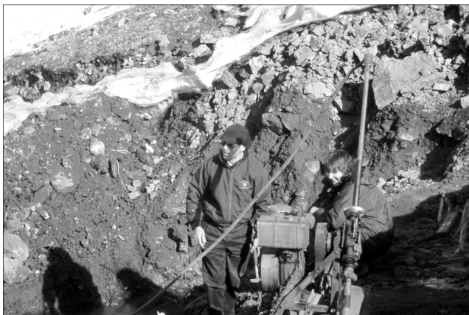
Figure 7. An X-ray drill capable of drilling AX core is pictured in trench 99-01 on the Horn property. Photo by J. Duke
