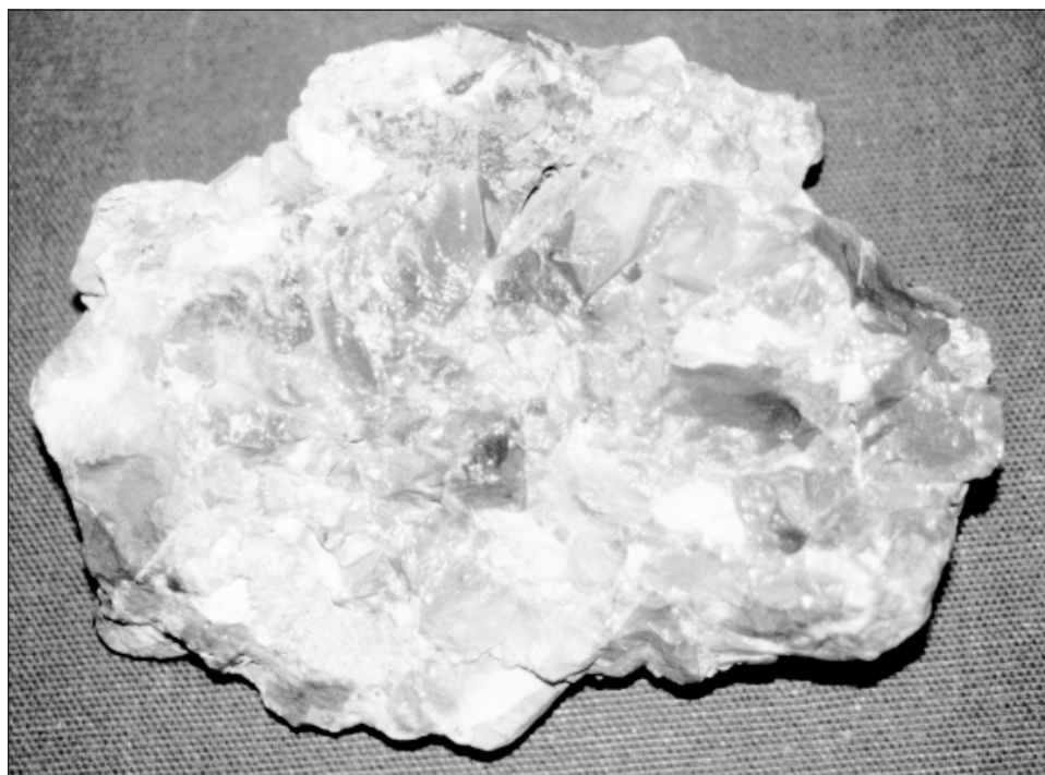
Figure 13. Quartz breccia with argillite and clay-altered intrusive fragments from the Harlan property of NovaGold Resources Inc.
