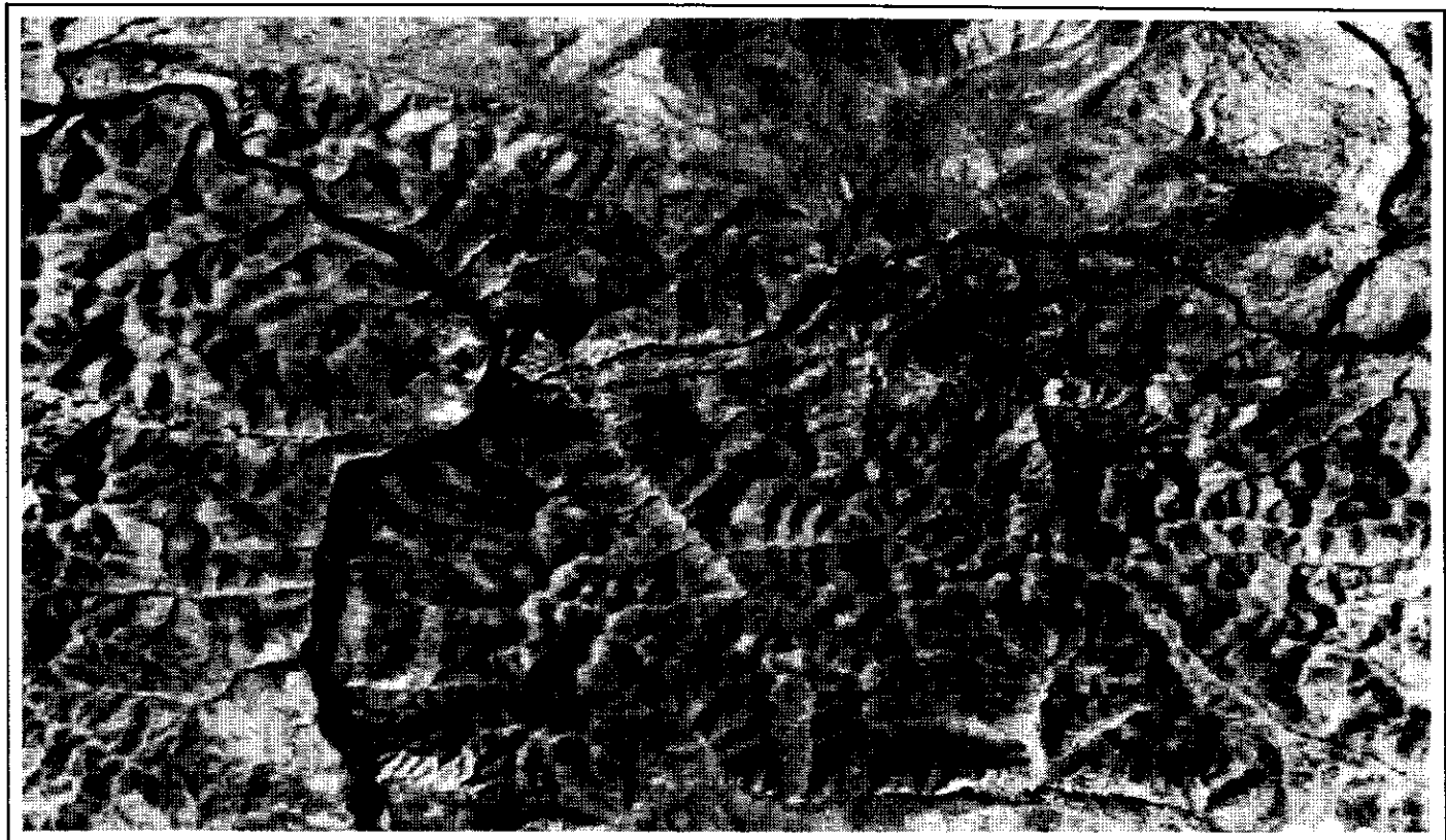
Figure 2a. NW area. Linearly contrast-stretched image of the TM Band 6 (thermal) data for the study area.
