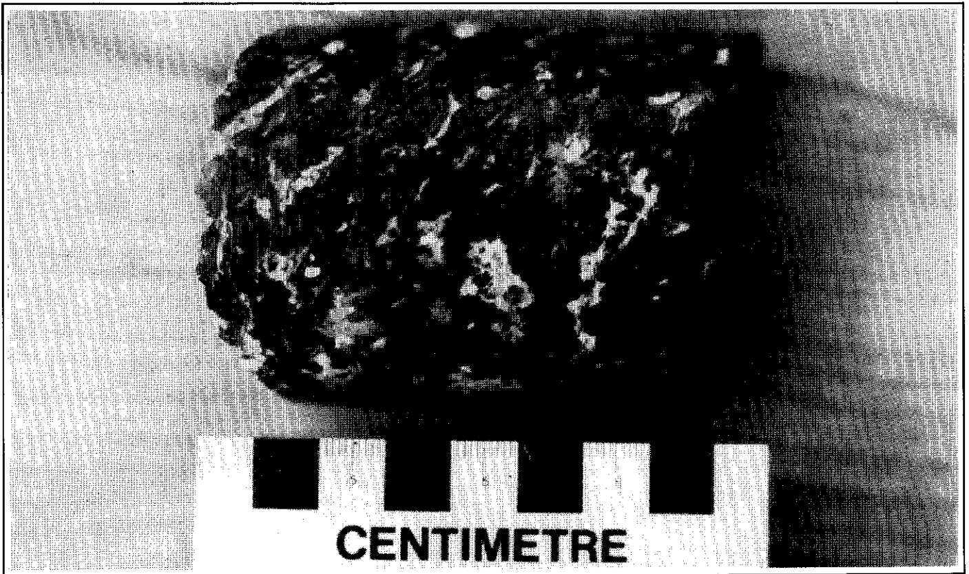
Figure 11. Drill core of welded vitric ash tuff from 123.3 m downhole in DDH 65. Mild eutaxitic texture is marked by partial flattening of pumice fragments (white).
