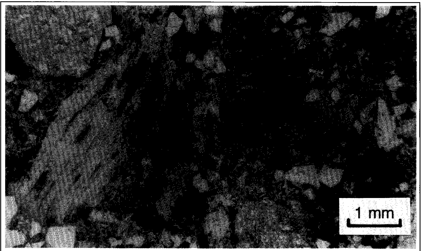
Figure 9. Thin section of CLP tuff (DDH 66 at 181.5 m downhole depth) under plane polarized light, showing quartz (white) and hydrothermally altered feldspar and rock fragments (mottled grey), pumice (lower left) and pyrite (black).
