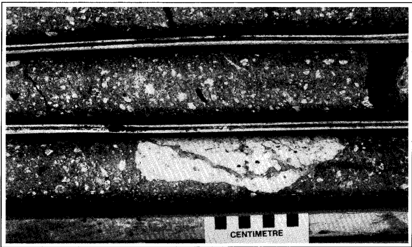
Figure 8. Drill core of CLP tuff with 18 cm long pumice block (immediately above scale) at a downhole depth of about 72 m in DDH 72.
