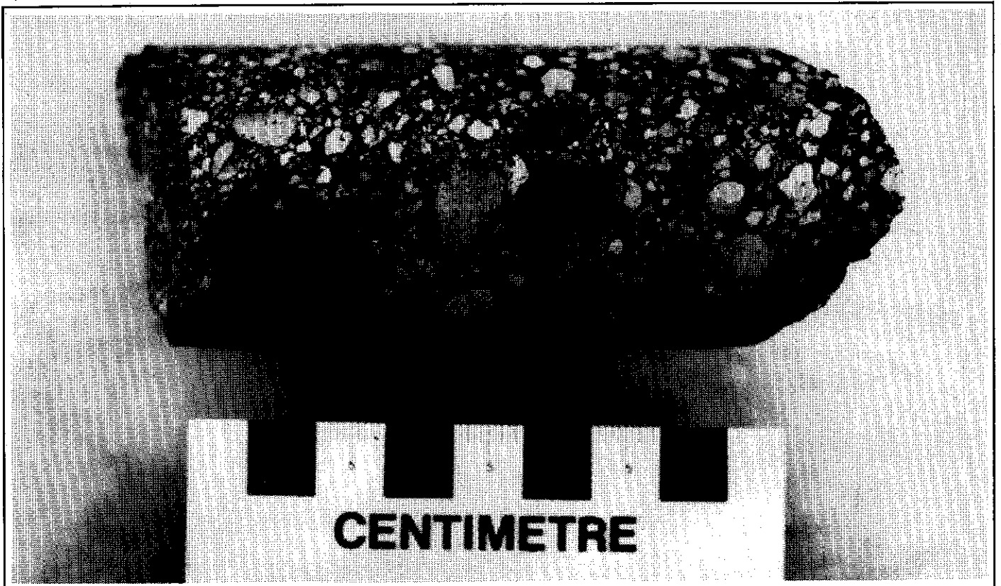
Figure 13. Drill core of basaltic lapilli tuff from a downhole depth of 307 m in DDH 82.
