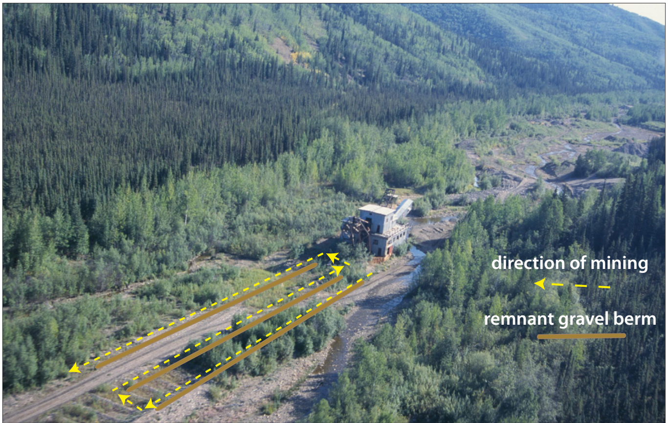
Figure 8. Reefs and berms of virgin gravel are often left behind as these barriers are sometimes required to maintain pond integrity. The photo above illustrates how these berms are created during the dredging process.
