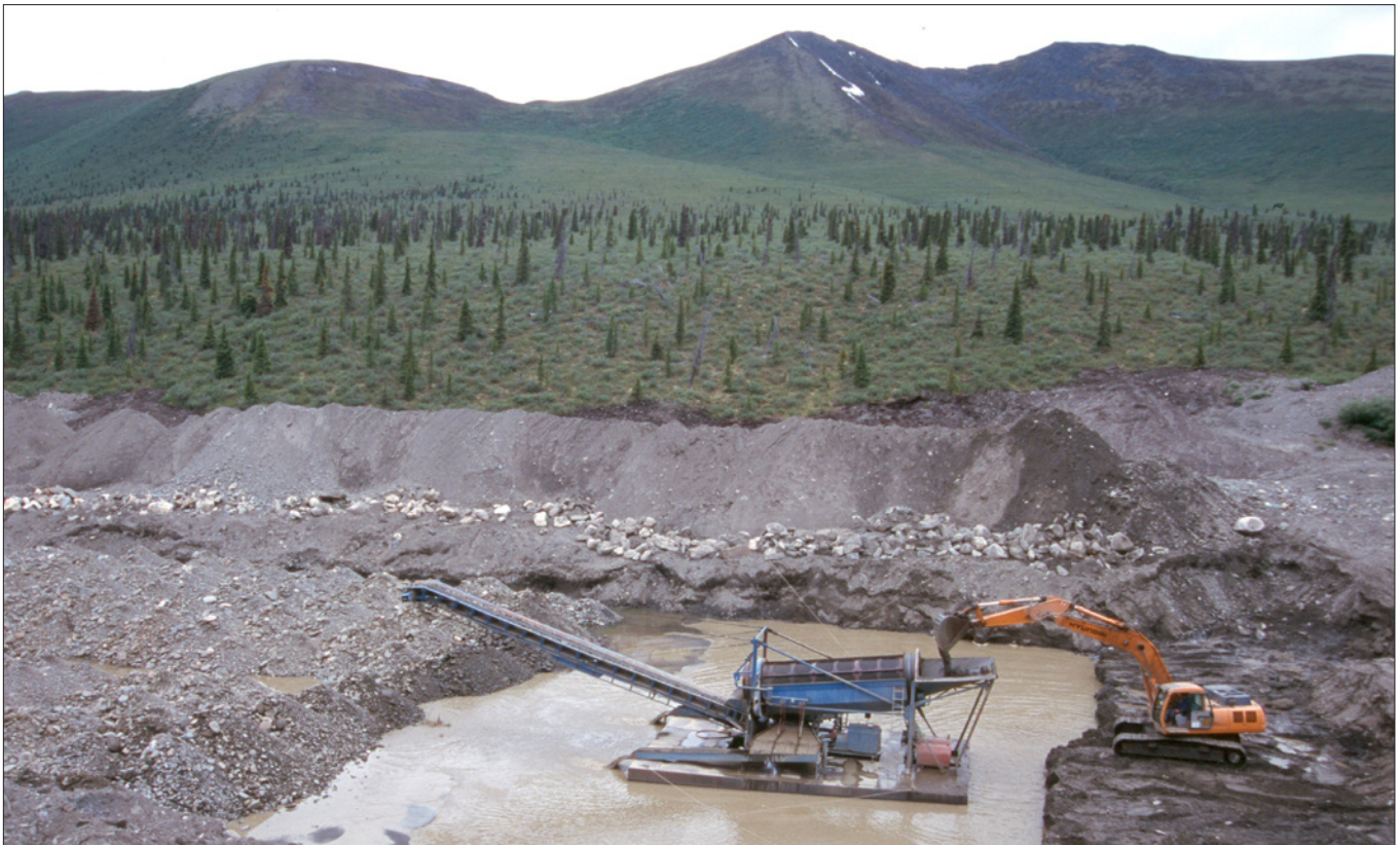
Figure 6. On Fourth of July Creek, economic placer gravels have been found beneath previously mined gravel layers. Newer mining technologies such as floating trommel wash plants have helped to overcome past difficulties such as mine pit drainage problems.
