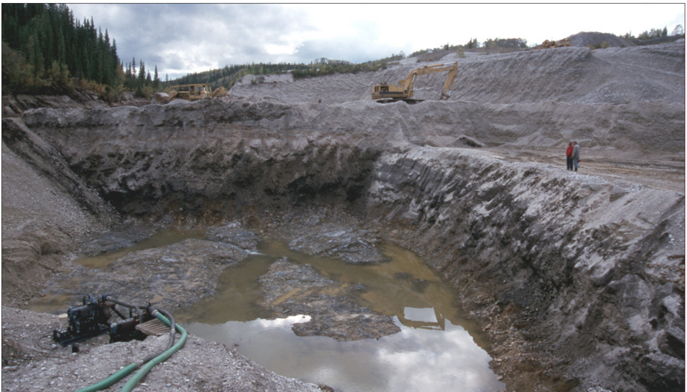
Figure 3. In the Klondike, human-made alluvial fans were often created during hydraulic mining of the high-level White Channel Gravel terraces, such as here on Last Chance Creek. In addition to containing sporadic, locally economic, concentrations of gold, these hydraulic fans locally buried virgin alluvial gravels and old timers' workings containing economic gold values.
