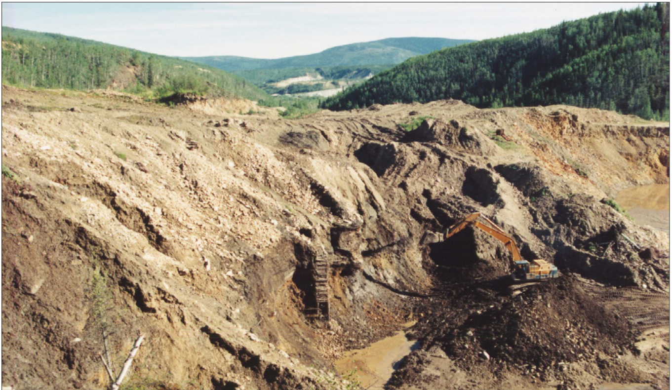
Figure 2. Buried channels of virgin gravel are occasionally discovered, having been initially obscured by bedrock reefs such as here on Bonanza Creek. Old timers often mined such high-grade material that even their tailings contain economic gold at today's prices.
