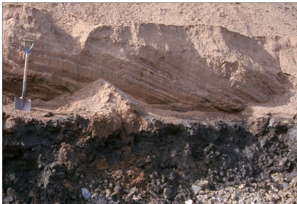
Figure 4. Dredge tailings are easily recognized by the inverted stratigraphy and unusually well-developed planar tabular cross-stratification. Gold values in these tailings are rarely economic, however, combined with pockets of virgin gravel in undulating bedrock, there may be a mineable technogenic placer deposit.
