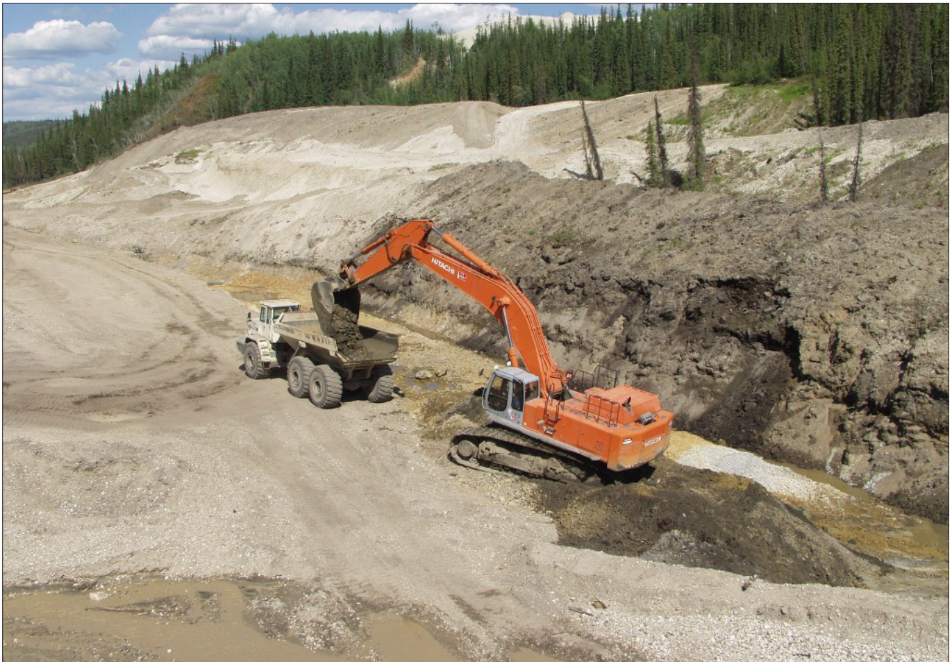
Loading pay gravel, Favron Enterprises Ltd., 2003.
