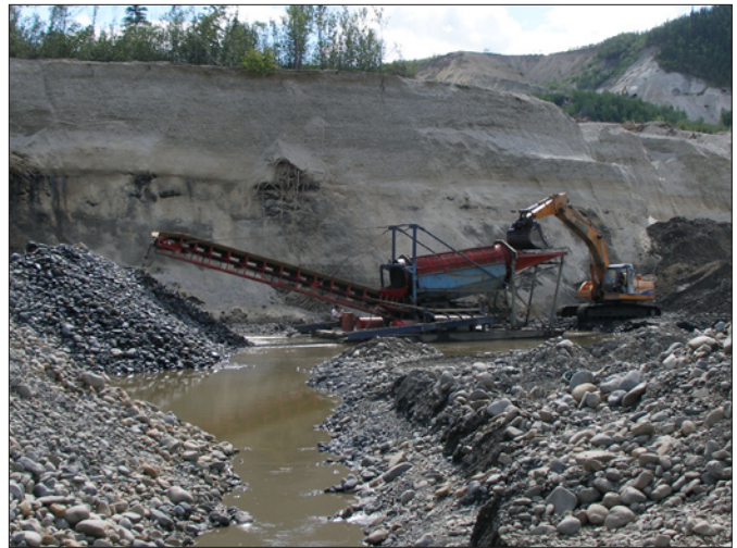
Gary Crawford's wash plant operating on the Klondike River at the base of Jackson Hill, 2006.
