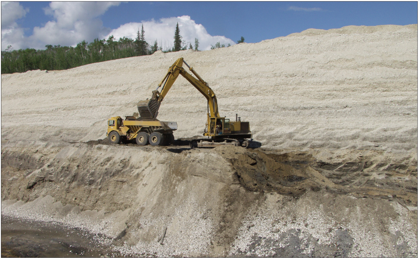
Stripping hydraulic tailings at Henry Gulch Placers' operation on Last Chance Creek, 2003.
