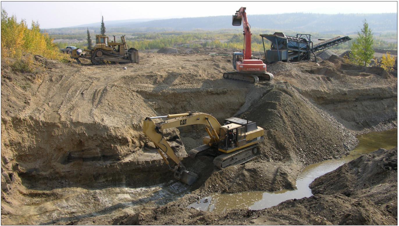
Kim Ferguson relaying pay gravel to wash plant at the mouth of Quartz Creek, 2004.
