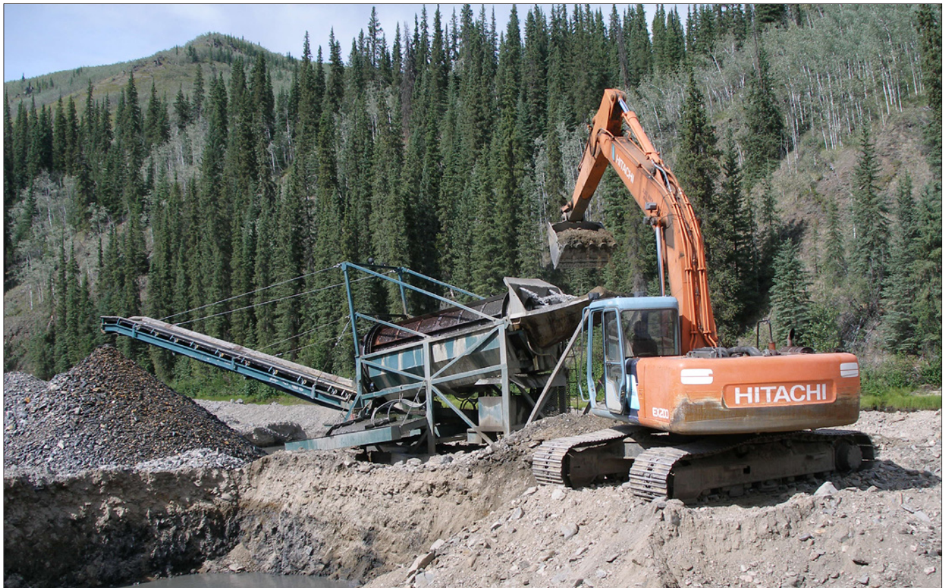
Feeding the wash plant at Dave McBurney's Indian River mine, 2006.
