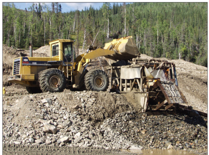
Sluicing pay gravel at Zdenek Bidrman's operation on Scroggie Creek, 2004.
