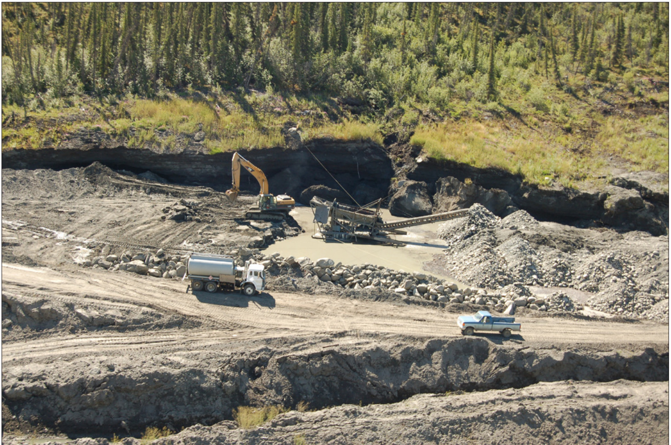
View of Tic Exploration's 5-foot-diameter trommel operating on the left limit of Gladstone Creek, 2006.
