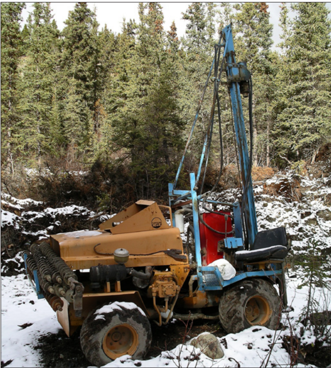
Sid McKeown's mobile drill for placer testing, Wolverine Creek, 2005.
