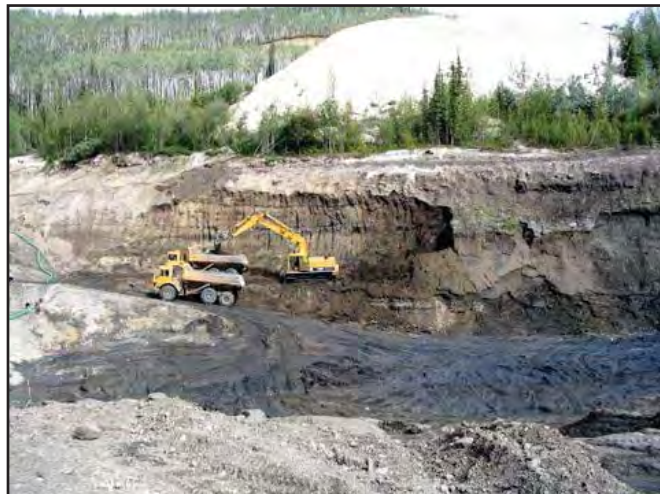
Stripping overburden at Tatra Ventures Hunker Creek operation in 2008.
