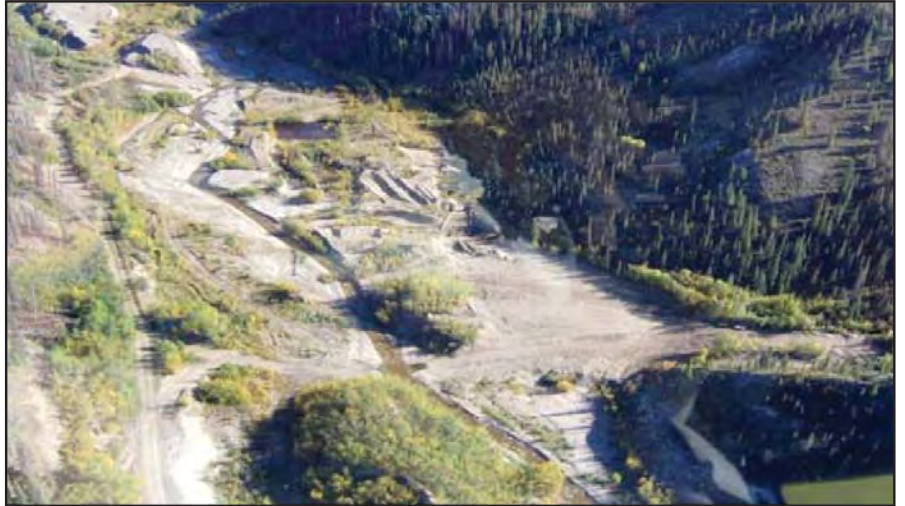
One site from which No Name Resources Inc. removed the abandoned debris remaining from many years of placer operations. The site was re-sloped and contoured in preparation for natural revegetation.
