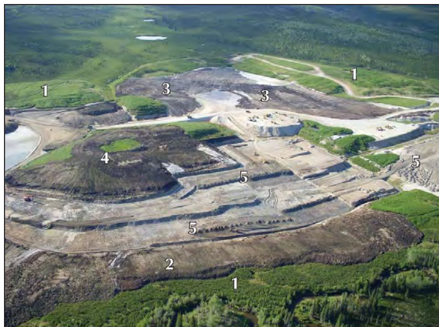
Placer mining continues at the Ross Mining operation next to reclaimed areas. Numbers 1 to 5 represent areas that have been reclaimed or are in the process of being reclaimed. Number 1 is the oldest and number 5 is the youngest.
