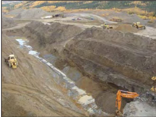
Fine Gold Resources Ltd. mining cut on the left limit bench of Eureka Creek in 2007.
