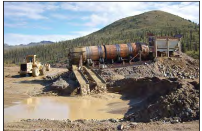
Johnson Exploration's trommel at their mining operation on Nansen Creek in 2007.
