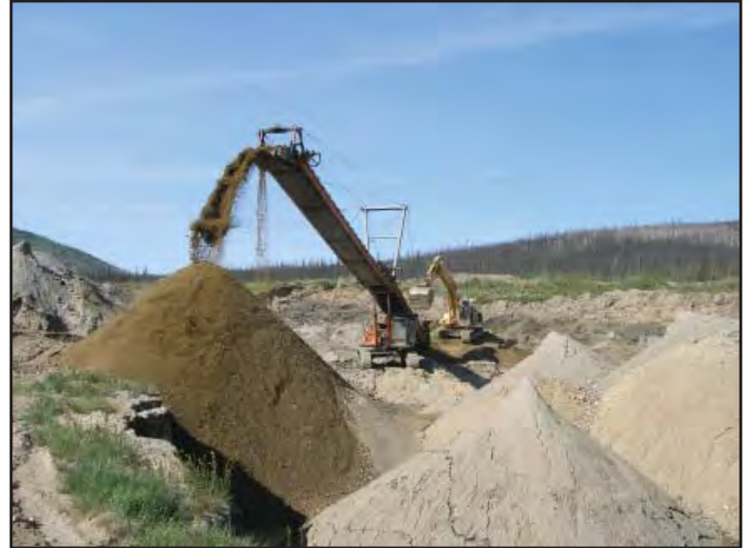
Adrian Hollis' Dominion Creek operation used a mobile conveyor mounted on a Hitachi EX450-LCH with an extension 'slinger' to strip overburden.
