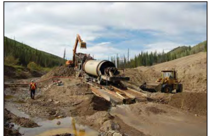
The trommel operated by Maisy Mae Mining on Maisy May Creek in 2008 was acquired from an operation on Anderson Creek in the Mayo Mining District. It featured a unique internal reverse-spiral which looped pay material back to a side sluice run.
