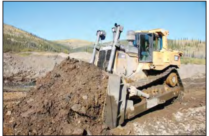
H.C. Mining acquired a new Caterpillar D9T for their mining operation on Henderson Creek in 2008. It turns on a dime and is very fuel-efficient.
