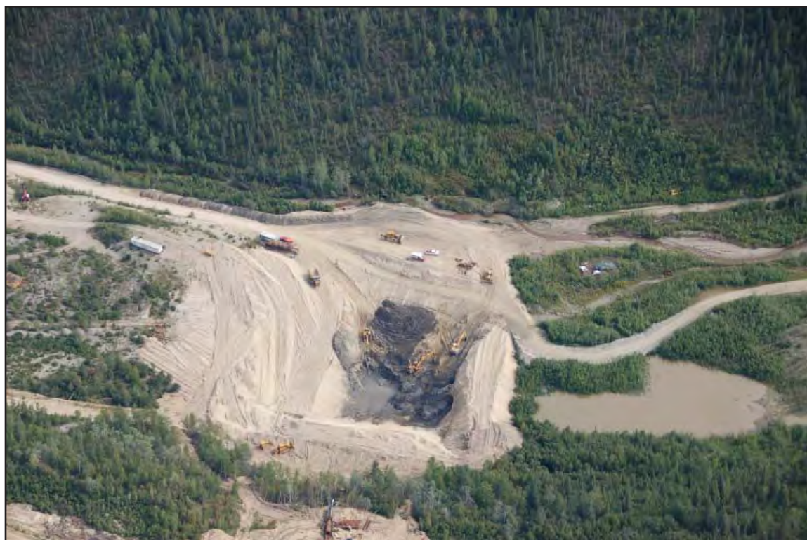
38945 Yukon Ltd.'s mining operation on the left limit of Eldorado, 2009. The wash plant can be seen at the bottom centre of the photo.
