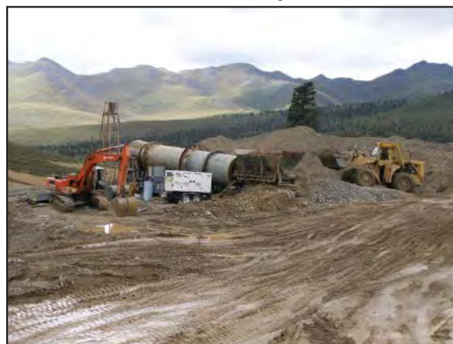
Nansen Gold Resources trommel at their mine on the East Fork of Nansen Creek in 2007.
