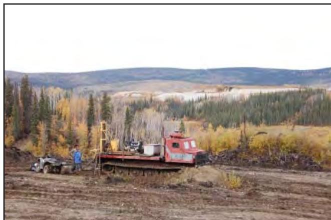
Last Chance Placers auger drilling on Last Chance Creek in 2008.
